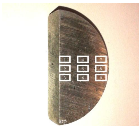
Figure 3. The scheme of microstructure parameters (Table 1) measurement on the cross-section—the numbered areas have dimensions 1034 \times 776 \mu\text{m} (magnification 100\times ).
