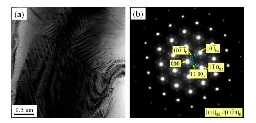
**Figure 6.** TEM micrographs of an as-rolled NiTi SMA sample subjected to aging: (**a**) Bright field image; (**b**) Diffraction pattern of (**a**).
