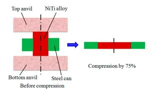
Figure 1. Schematic diagram of NiTi SMA sample subjected to local canning compression.
