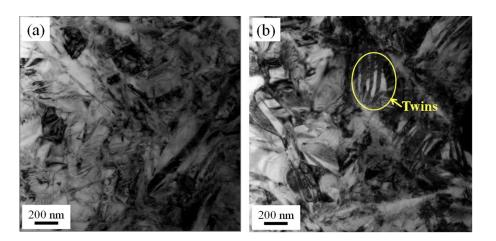
**Figure 8.** TEM micrographs of an as-rolled NiTi SMA sample subjected to SPD and subsequent aging: (a) Bright field image showing martensite morphology; (b) Bright field image showing the existence of martensite twins.
