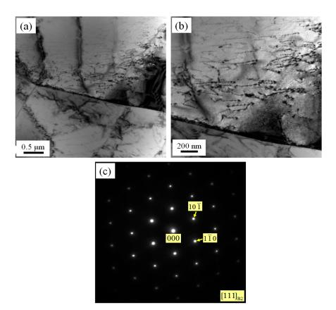
Figure 2. TEM micrographs of as-rolled NiTi SMA sample: (a) Bright field image (low magnification);(b) Bright field image (high magnification); (c) Diffraction pattern of (b).
