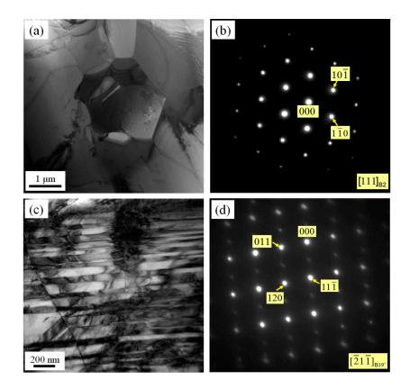
**Figure 9.** TEM micrographs of a solution-treated NiTi SMA sample subjected to SPD and subsequent aging: (a) Bright field image showing B2 austenite phase; (b) Diffraction pattern of (a); (c) Bright field image showing B19' martensite phase; (d) Diffraction pattern of (c).
