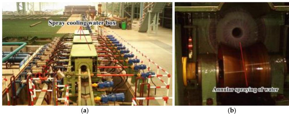
**Figure 3.** Arrangement of water boxes and its operating state (a) arrangement of spray water boxes; (b) operating state of spraying water.
