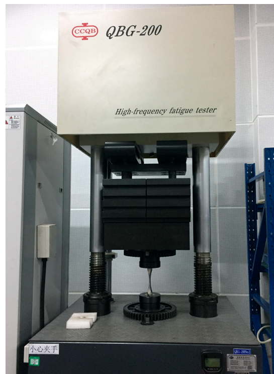
Figure 6. Setup of the fatigue experiments.
