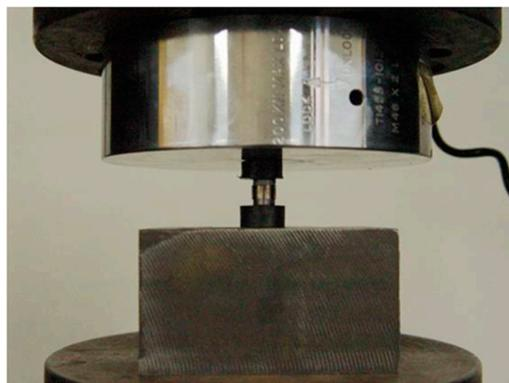
**Figure 1.** Photograph of NiTi shape memory alloy (SMA) tube undergoing radial loading test.
