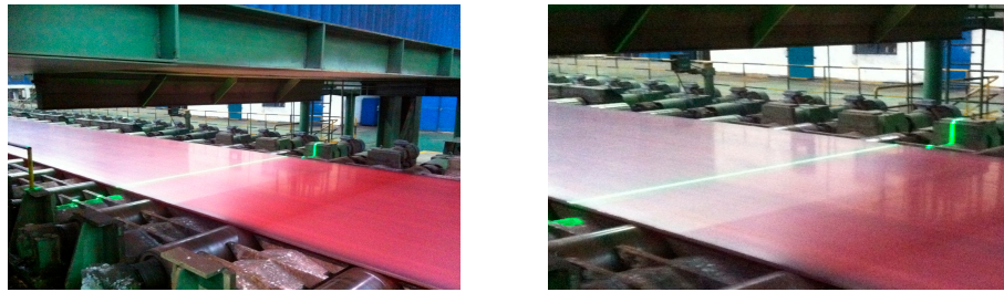
Figure 2. Surface inspection system of hot rolled steel plates with green linear laser lighting.
