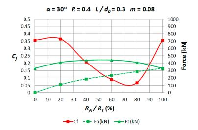
**Figure 11.** Damage factors ( $C_f$ ) and forces versus  $R_A/R_T$ .
