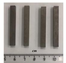
**Figure 7.** Pulsed electrospark deposition (PED) electrodes obtained using force self-propagating high-temperature synthesis (SHS)-pressing technology in a Ti–C–Co–Ca<sub>3</sub>(PO<sub>4</sub>)<sub>2</sub>–Ag–Mg system.
