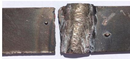
**Figure 8.** Type of sample failure found during tensile tests; failure due to initial rupture in the HAZ area.
