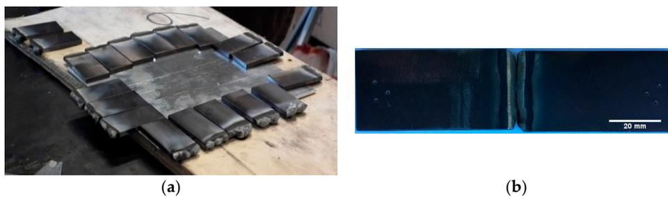
**Figure 3.** Test specimens after Nickel filler metal deposition: (a) welded Nickel bead to chamfer edge; and (b) re-chamfered edges after Nickel deposition.
