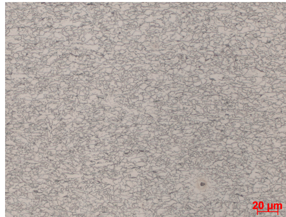
Figure 1. Microstructure of high strength steel B550CL.
