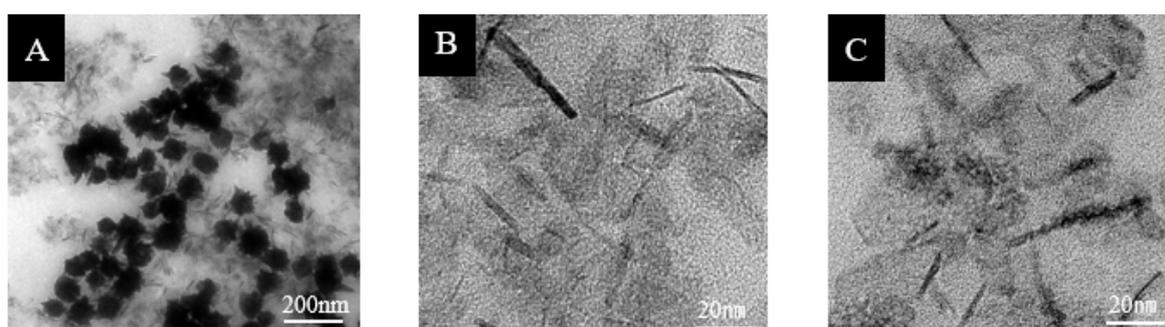
**Figure 2.** Field emission transmission electron microscopy (FE-TEM) images of synthesized nickel particle: (A) no addition of PVP; (B) PVP of 1 g; (C) PVP of 2 g.
