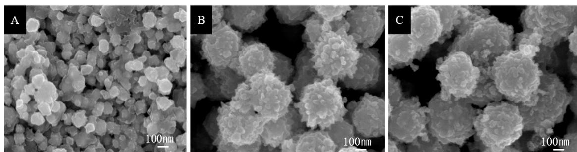
**Figure 1.** Field emission scanning electron microscopy (FE-SEM) images of reduced nickel particle: (A) NaOH of 10 g; (B) NaOH of 12.5 g; (C) NaOH of 15 g.
