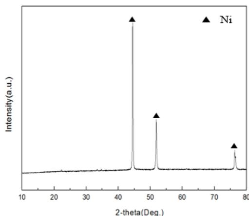
Figure 3. X-ray diffraction (XRD) pattern of synthesized nickel particle.
