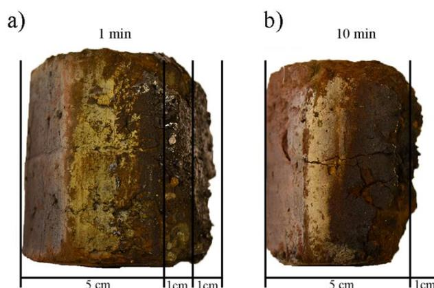
**Figure 6.** Photographs of the briquettes of Table 4 after contact with hot metal at 1350 °C for (a) 1 min, and (b) 10 min [30].
