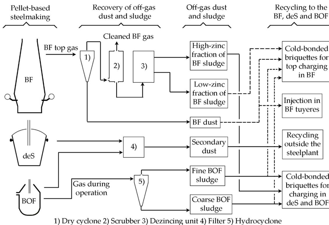
**Figure 8.** Illustration of the holistic view on recycling of off-gas dust within the integrated steel plant.
