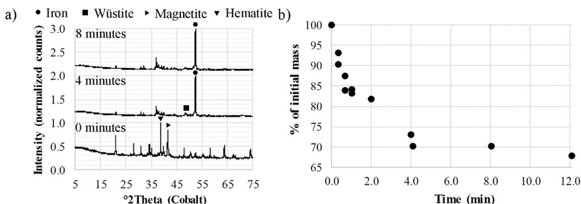
**Figure 7.** (a) Diffractograms of pellets with 100% peaks of the iron phases denoted; (b) mass loss of the pellets with respect to the time of contact with hot metal at 1350 °C [30].
