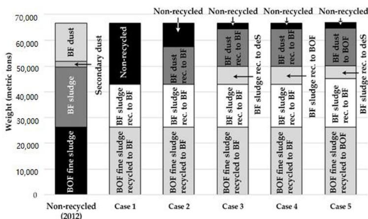
**Figure 1.** Annual generation of residues not recycled as of 2012, as well as recycling considered in cases 1 through 5. All weights are given in dry weights.
