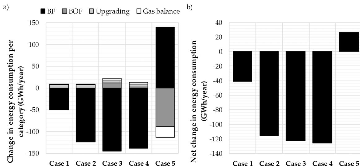
**Figure 3.** Results of the process integration analyses: (a) Change in energy used in each process; (b) net change in energy consumption.
