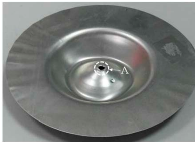
Figure 18. Photo of electromagnetic high-speed impact fracture specimen.
