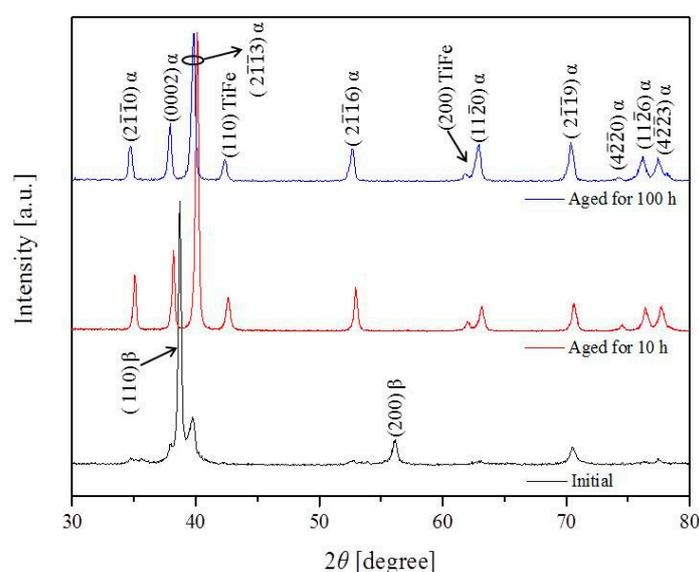
**Figure 3.** XRD patterns of initial Ti-5Al-3.5Fe alloy and alloy after aging at 500 °C for 10 or 100 h.
