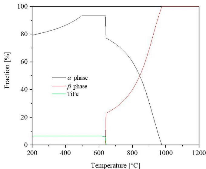
**Figure 1.** Equilibrium phase information of Ti-5Al-3.5Fe alloy used in this work as a function of temperature, showing possible phases and their fraction; this result was obtained by JMatPro-v8 calculation with Ti database.
