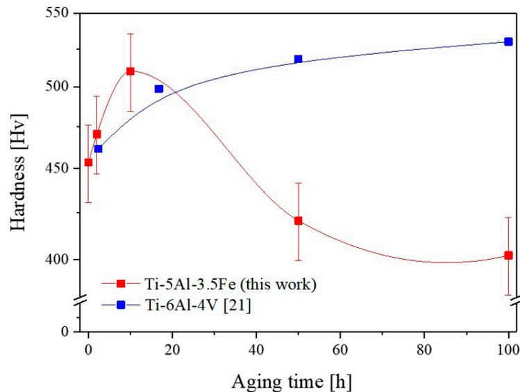
**Figure 6.** Variation in average hardness with aging time; the value at aging time = 0 h indicates the hardness for the initial material. Error bars indicate the standard deviations. A result of Ti-6Al-4V [21] is presented for comparison.
