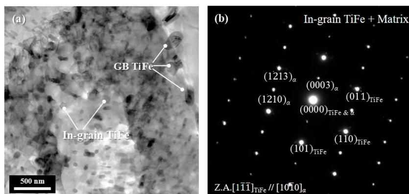
**Figure 5.** TEM analysis results of Ti-5Al-3.5Fe alloy after aging for 100 h. (a) Bright-field image and (b) corresponding diffraction patterns.
