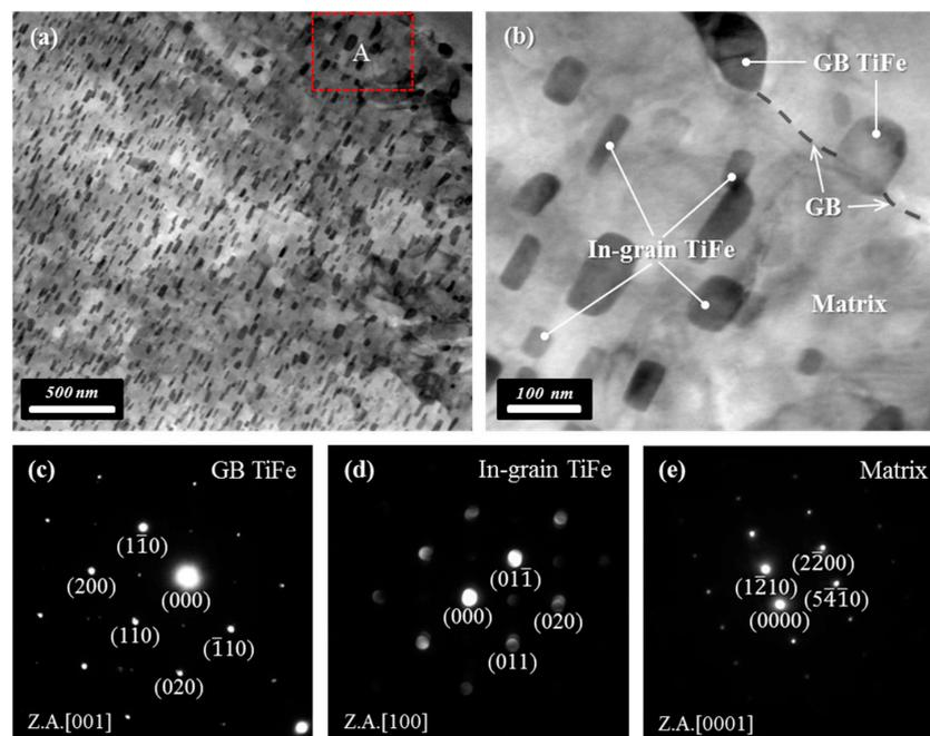
**Figure 4.** TEM analysis results of Ti-5Al-3.5Fe alloy after aging for 10 h. (a) Bright-field image, (b) magnification of the area A indicated in (a), and (c–e) diffraction patterns of three important phases observed in (b).
