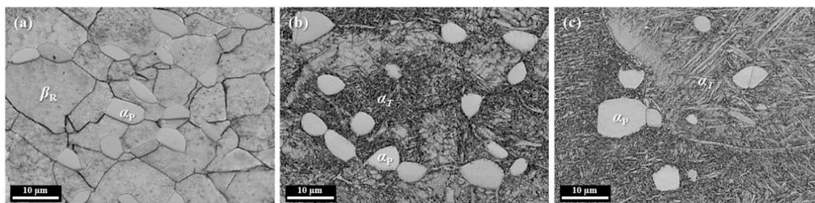
**Figure 2.** SEM images of Ti-5Al-3.5Fe alloy. (a) Initially, (b) after aging for 10 h, and (c) after aging for 100 h, at 500 °C;  $\alpha_p$ : primary  $\alpha$  phase;  $\beta_R$ : retained  $\beta$  phase;  $\alpha_T$ :  $\alpha$  phase transformed from retained  $\beta$  phase.
