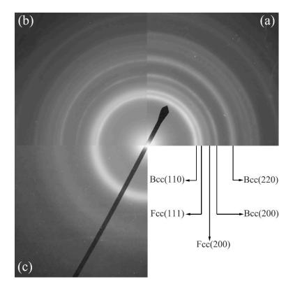
**Figure 7.** The SAD patterns of resultant phases formed in the Ni<sub>51</sub>Nb<sub>19</sub>Mo<sub>30</sub> nano-multiple-metal-layers [71] (a) at as-deposited state, after being irradiated to a dose of (b)  $1 \times 10^{15}$  Xe<sup>+</sup>/cm<sup>2</sup> and (c)  $5 \times 10^{15}$  Xe<sup>+</sup>/cm<sup>2</sup>.
