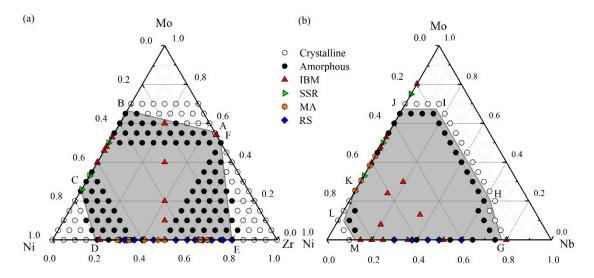
**Figure 4.** The glass formation region (the central area) derived from molecular dynamics (MD) simulation with various experimental data for (**a**) a Ni-Zr-Mo system [56] and (**b**) a Ni-Nb-Mo system [55].
