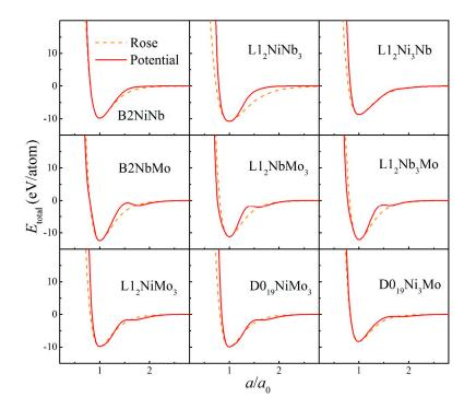
**Figure 1.** Total energies calculated from interatomic potential (*Red solid line*) and corresponding Rose equation [65] (*Orange dashed line*) as a function of lattice constant for various compounds in the Ni-Nb-Mo system.
