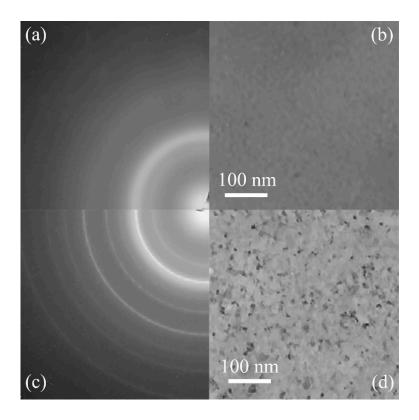
**Figure 8.** The SAD patterns and corresponding bright field image of the  $(\mathbf{a},\mathbf{b})$  (NiZr)<sub>60</sub>Mo<sub>40</sub> and  $(\mathbf{c},\mathbf{d})$  (NiZr)<sub>40</sub>Mo<sub>60</sub> nano-multiple-metal-layers [72] after irradiation with a dose of  $7 \times 10^{15}$  Xe<sup>+</sup>/cm<sup>2</sup>.
