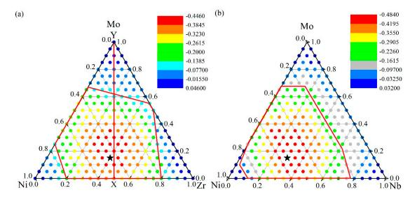
**Figure 6.** The formation energy difference between the solid solution and amorphous phase for (a) Ni-Zr-Mo system [56], and (b) Ni-Nb-Mo system [55]. The quantitative energy scale for dots with different colors are presented for the respective systems.
