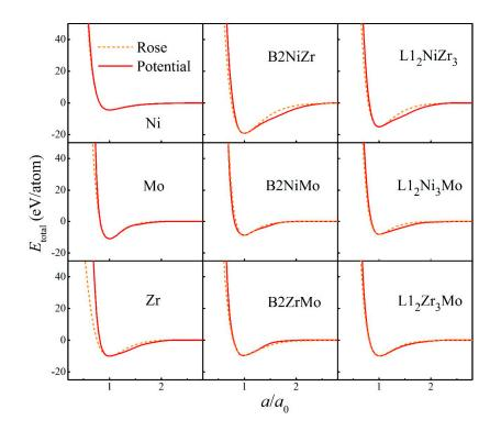
**Figure 2.** Total energies calculated from interatomic potential (*Red solid line*) and corresponding Rose equation [65] (*Orange dashed line*) as a function of lattice constant for pure metals as well as B2 and L1<sub>2</sub> compounds in the Ni-Zr-Mo system.
