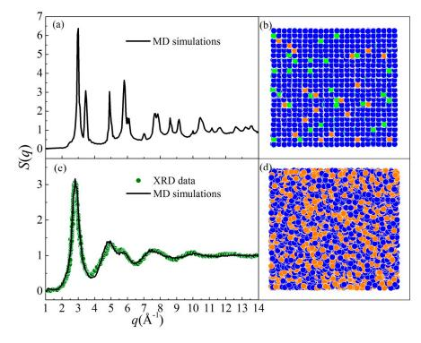
**Figure 3.** The structure factor (*S*(*q*)) and projection of atomic positions for (**a**,**b**) the crystalline state (Ni<sub>90</sub>Zr<sub>5</sub>Mo<sub>5</sub>) and (**c**,**d**) the amorphous state (Ni<sub>64</sub>Zr<sub>36</sub>), respectively [56]. The XRD data [73] for Ni<sub>64</sub>Zr<sub>36</sub> MGs are also presented and marked as olive dots. Blue solid circles are for Ni, orange solid circles for Zr, and yellow solid circles for Mo.
