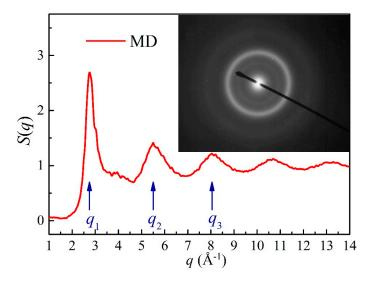
**Figure 5.** The structure factor S(q) of the Ni<sub>52</sub>Nb<sub>35</sub>Mo<sub>13</sub> alloy derived from MD simulation [55] and the corresponding selected area diffraction (SAD) patterns [71]. The  $q_1$ ,  $q_2$  and  $q_3$  represent the first, second and third peak positions of the structure factor S(q).
