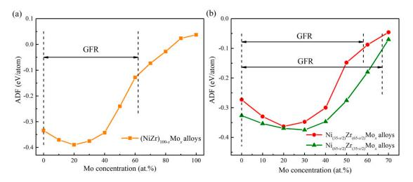
**Figure 9.** The amorphization driving force (ADF) for the  $(NiZr)_{100-x}Mo_x$  alloy [56] as shown by the XY line in Figure 6 (**a**), as well as the ADF for the  $Ni_{(35-x/2)}Zr_{(65-x/2)}Mo_x$  and  $Ni_{(65-x/2)}Zr_{(35-x/2)}Mo_x$  alloys (**b**).
