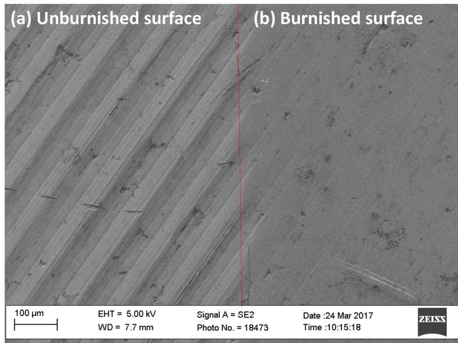
**Figure 11.** SEM photo of surface topography (a) before and (b) after burnishing at  $F = 1650$  N,  $f = 300$  mm/min, and  $S = 0.10$  mm.
