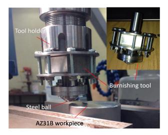
Figure 2. Experimental setup of the burnishing.
