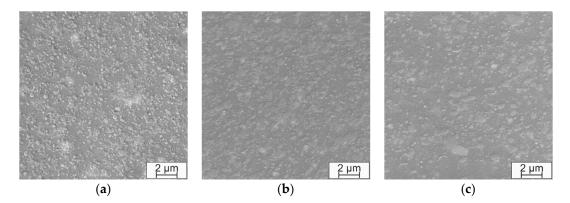
**Figure 3.** SEM images of AMCs produced by means of high-energy ball milling, hot isostatic pressing and extrusion in the T4 condition; matrix alloy AA2017; reinforced with SiC particles: (**a**) 15 vol %  $\beta$ -phase with size < 0.2  $\mu$ m; (**b**) 15 vol %  $\alpha$ -phase with size < 1  $\mu$ m; and (**c**) 10 vol %  $\alpha$ -phase with size < 1  $\mu$ m.
