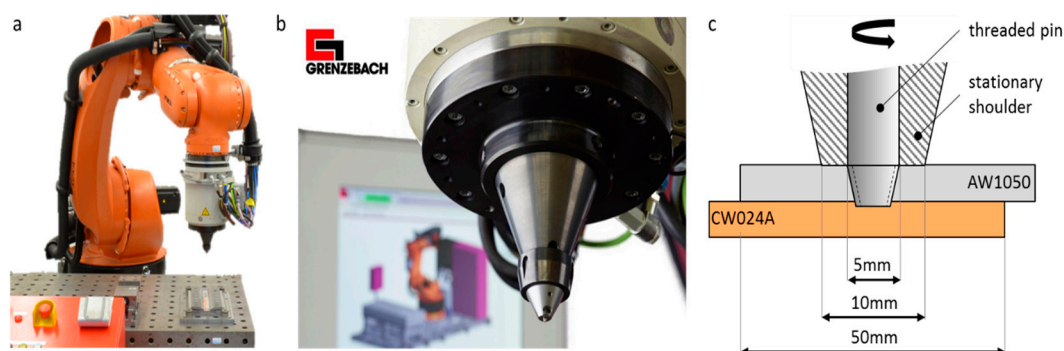
Figure 1. Process setup: (a) Robotic friction stir welding (FSW) system (Grenzebach); (b) Stationary shoulder tool; (c) Schematic illustration of the tool and joint configuration.
