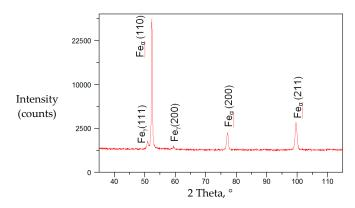
**Figure 6.** X-ray diffraction of the butt weld made in steel S700MC using the MAG method and a linear energy of 8 kJ/cm.
