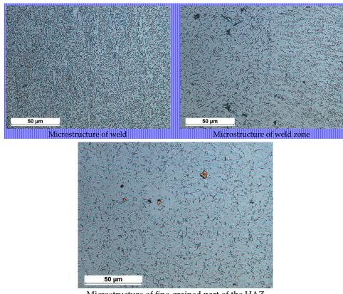
Microstructure of fine-grained part of the HAZ
