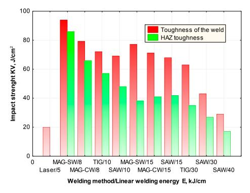
**Figure 10.** Effect of welding method and heat input on the toughness of the welded joints made of steel S700MC.
