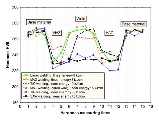
**Figure 8.** Effect of welding method and input heat on the hardness on the cross section of the S700MC welded joints.
