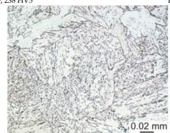
Cooling times  $t_{8/5}$  = 87.84 s; ferrite + bainite structure; 192 HV5
