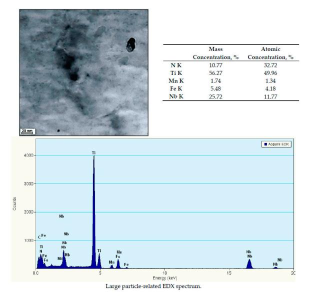
**Figure 2.** Precipitation of carbonitride (Ti,Nb)(C,N) with numerous small dispersive precipitates corresponding to the hardening of steel.
