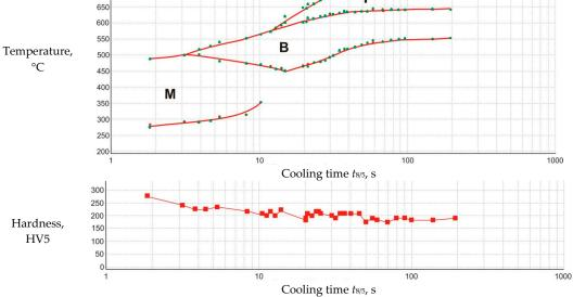
**Figure 4.** Chart of structural changes in the steel S700MC in terms of welding CCT-W together with complementary graph on the distribution of hardness as a function of the cooling time  $t_{8/5}$ .
