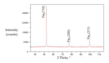
**Figure 7.** X-ray diffraction of the butt weld made in steel S700MC using laser beam welding and a linear energy of 5 kJ/cm.
