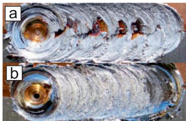
**Figure 23.** Comparison between a weld with defects (a) and one without defects (b).
