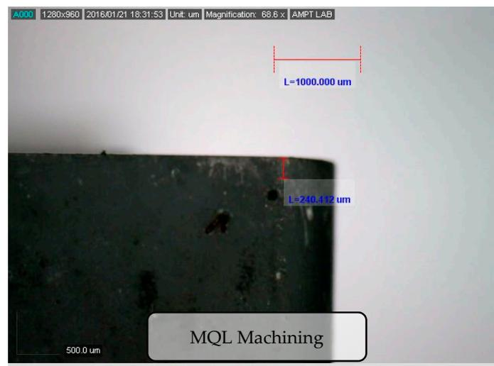
Figure 6. No built-up edge (Experiment no-11).
