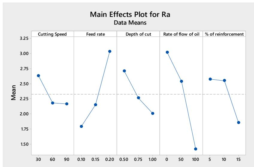
**Figure 4.** Mean effects plot for surface roughness.
