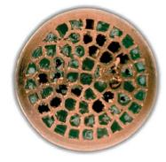
**Figure 18.** UniPore structure with 46.7% porosity filled with phase change material (PCM). Reproduced from [1], with permission from Elsevier, 2015.
