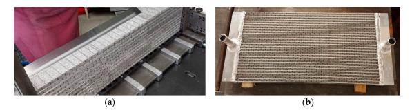
**Figure 19.** (a) Assembly of a heat exchanger with AlSi1 short-fiber structures by stacking flat tubes and AlSi1 short-fiber structures. (b) Finished heat exchanger with AlSi1 short-fiber structure, total fiber structure volume 6.7 L, core dimensions 600 mm  $\times$  316 mm  $\times$  45 mm.
