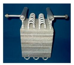
**Figure 20.** Photography of latent heat storage (without housing) before filling with PCM. Total fiber structure volume 8 L, dimensions of the fiber structure 200 mm  $\times$  200 mm  $\times$  200 mm.
