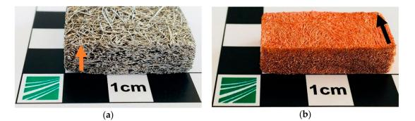
**Figure 4.** Photography of (**a**) AlSi1 short-fiber structure made from short metal fibers and (**b**) photography of copper long-fiber structure made from endless copper fibers. Arrows indicate the normal vector of the isotropic plane.
