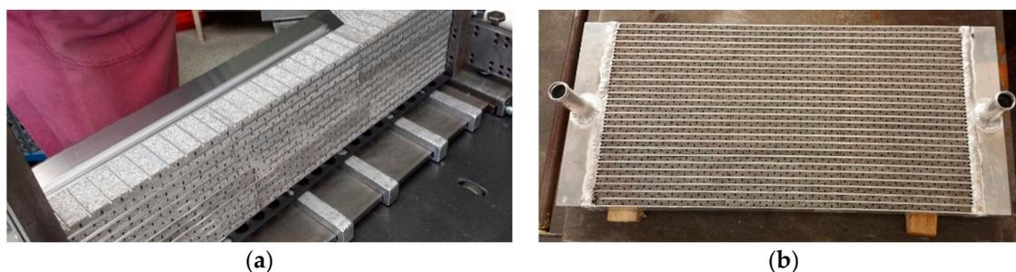
**Figure 19.** (a) Assembly of a heat exchanger with AlSi1 short-fiber structures by stacking flat tubes and AlSi1 short-fiber structures. (b) Finished heat exchanger with AlSi1 short-fiber structure, total fiber structure volume 6.7 L, core dimensions 600 mm × 316 mm × 45 mm.
