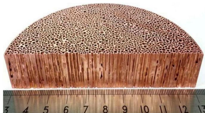
**Figure 1.** Section of a lotus-type porous copper ingot. Reproduced from [2], with permission from Elsevier, 2015.
