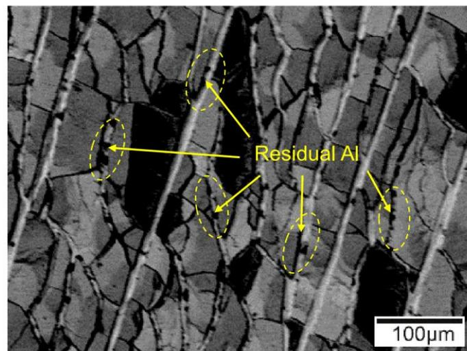
**Figure 10.** Peeling surface morphology (BSE image) of the Cu/Al clad sheet with a thickness of 5 mm after multi-pass rolling (Cu side).
