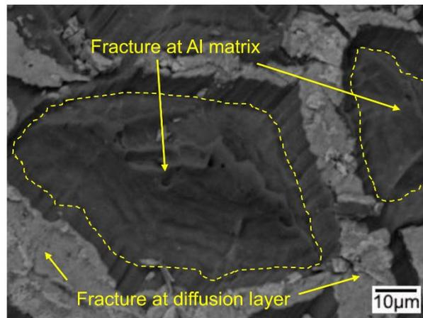
**Figure 17.** Peeled surface morphology (BSE image) of the Cu/Al clad sheet with a thickness of 3 mm after multi-pass rolling and annealing (Al side).
