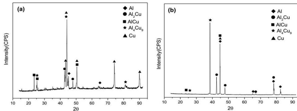
**Figure 4.** XRD pattern of the peeled surface for the as-cast Cu/Al clad sheet: (a) Cu side and (b) Al side.
