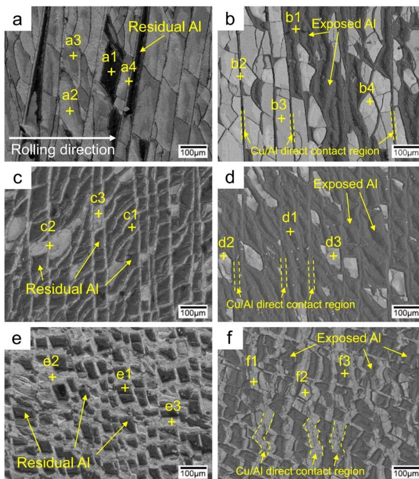
**Figure 11.** Peeled surface morphology (BSE image) of the Cu/Al clad sheets with thicknesses of 7 mm after multi-pass rolling and annealing (a,b), 5 mm (c,d) and 3 mm (e,f). (a,c,e: Cu side; b,d,f: Al side).
