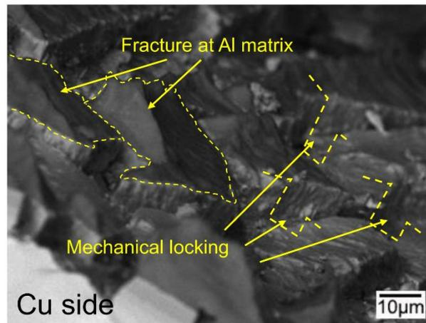
**Figure 15.** Peeled surface morphology (BSE image) of the Cu/Al clad sheet with a thickness of 7 mm after multi-pass rolling (Cu side).
