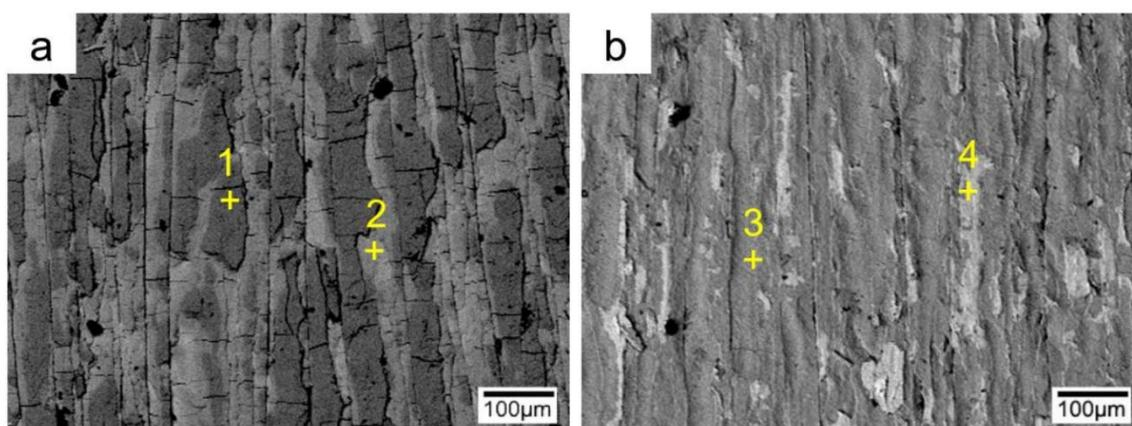
**Figure 8.** Peeled surface morphology (BSE image) and EDS results of the as-cast Cu/Al clad sheet: (a) Cu side and (b) Al side.
