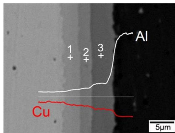
**Figure 3.** Microstructure (BSE image) of the as-cast Cu/Al clad sheet interface.
