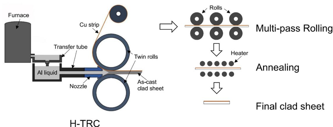
**Figure 1.** Schematic illustration of the fabrication process for Cu/Al clad sheet.
