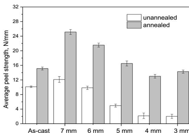
**Figure 7.** The average peel strength of the Cu/Al clad sheets under different conditions: H-TRC, multi-pass rolling, and annealing.
