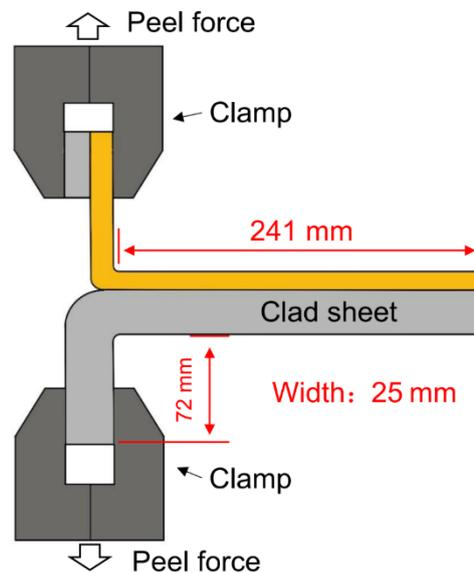
**Figure 2.** Test specimen and method of peel testing the clad sheets.
