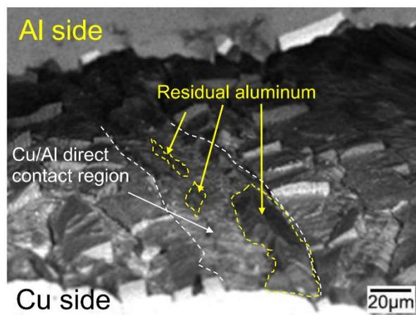
**Figure 16.** Peeled surface morphology (BSE image) of the Cu/Al clad sheet with a thickness of 3 mm after multi-pass rolling (Cu side).
