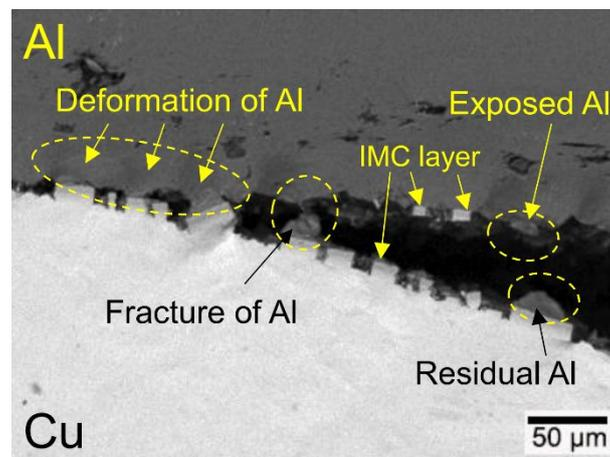
**Figure 14.** The cross section image (BSE image) of the fractured clad sheet with the rolled thickness of 5 mm.
