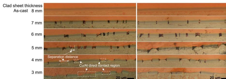
**Figure 5.** Interfacial microstructure of the Cu/Al clad sheets with different thicknesses after multi-pass rolling (left side) and annealing (right side).
