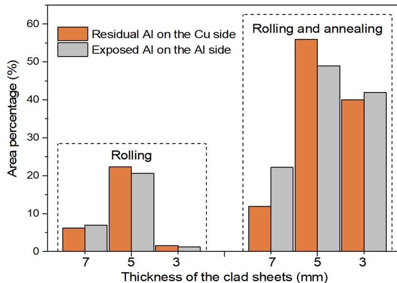
**Figure 12.** Areas percentage of the residual Al on the Cu side and exposed Al on the Al side with the clad sheet thickness reduction.
