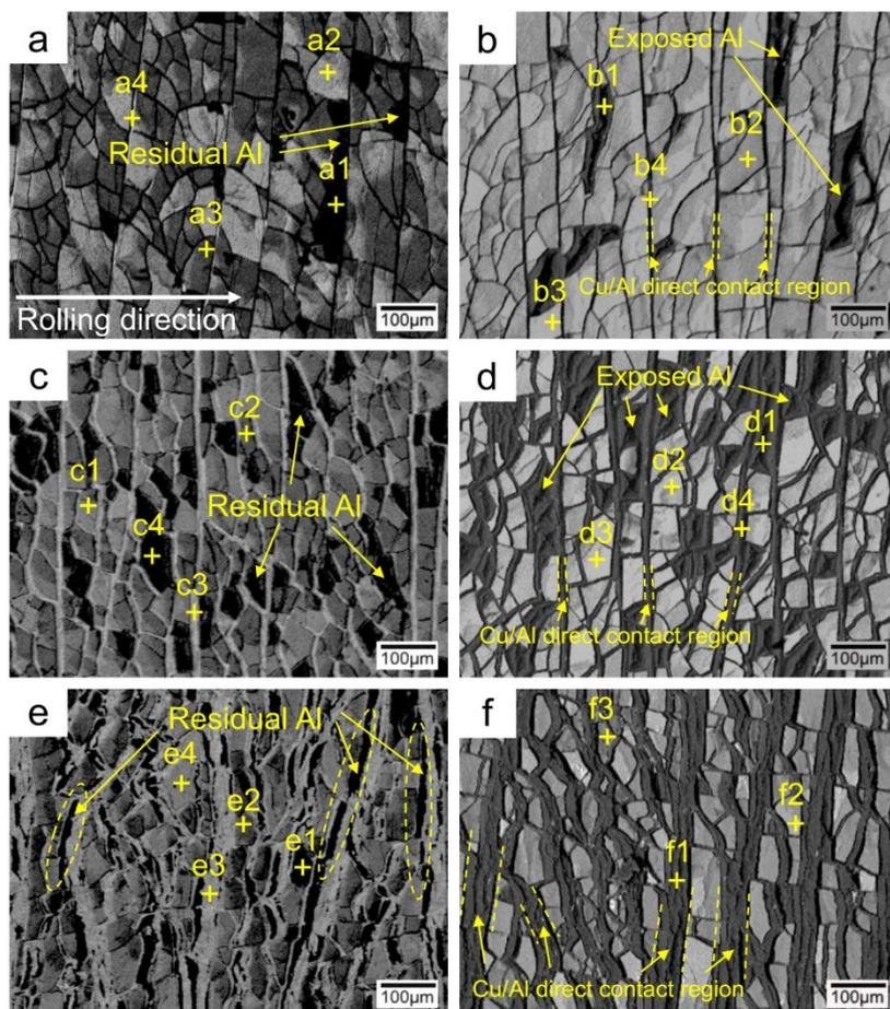
**Figure 9.** Peeled surface morphology (BSE image) of the Cu/Al clad sheets after multi-pass rolling with thicknesses of 7 mm (a,b), 5 mm (c,d) and 3 mm (e,f). (a,c,e: Cu side; b,d,f: Al side).
