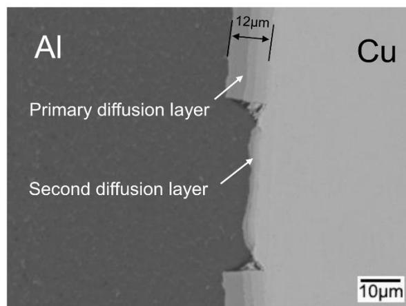
**Figure 6.** Microstructure (BSE image) of the Cu/Al clad sheet interface after multi-pass rolling and annealing (clad sheet thickness: 4 mm).
