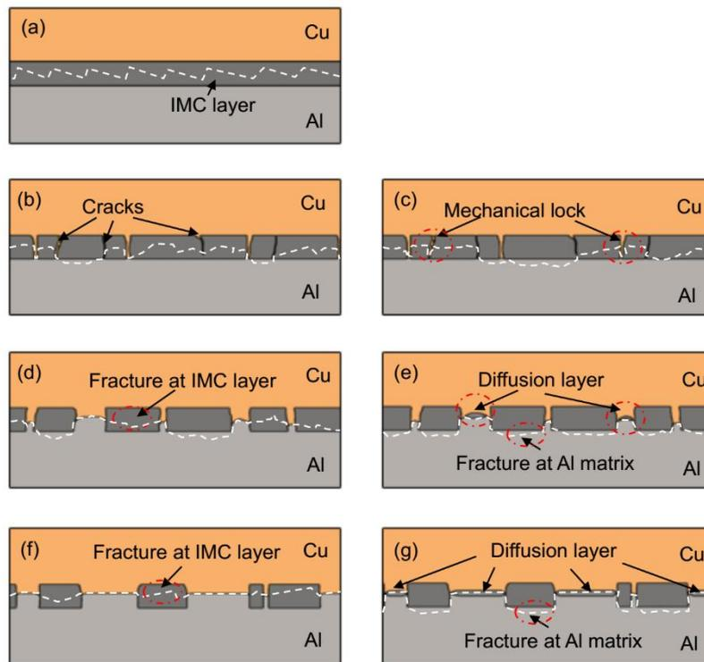
**Figure 13.** The schematic diagram of the bonding mechanism of Cu/Al clad sheets for rolling and annealing processes. (a) as-cast, (b) thickness of 7 mm after rolling, (c) thickness of 7 mm after rolling and annealing, (d) thickness of 5 mm after rolling, (e) thickness of 5 mm after rolling and annealing, (f) thickness of 3 mm after rolling, and (g) thickness of 3 mm after rolling and annealing.
