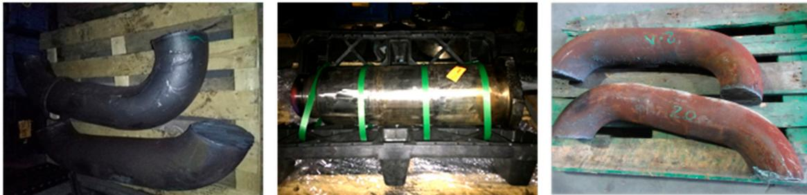
**Figure 1.** Left to right, samples A, B and C. **Sample A:** Two R4 chain link halves; **Sample B:** R4 Chain accessory; **Sample C:** Two R5 chain link halves.
