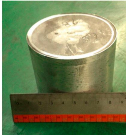
**Figure 1.** Macrograph of the fabricated semisolid billet of the nano-sized SiCp/7075 composite via rheoforming of the semisolid slurry prepared by ultrasonic-assisted semisolid stirring (UASS).
