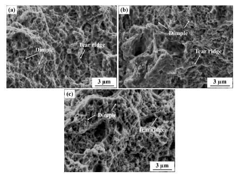
**Figure 11.** SEM images of tensile fractured surfaces of different heat treatment samples under the strain rate of 500 s<sup>-1</sup>: (a) B1; (b) B3; (c) Q&T.
