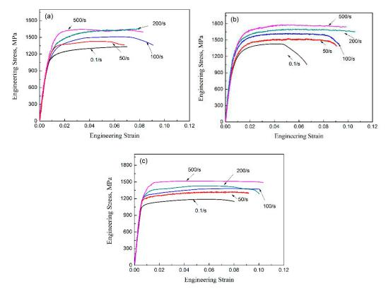
**Figure 9.** Engineering stress-strain curves of the quasi-static and the dynamic tensile tests of (**a**) B3, (**b**) B3, and (**c**) Q&T treatment samples.
