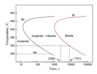
Figure 12. Time-temperature-transformation (TTT) curve of the investigated steel.
