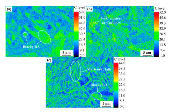
Figure 5. Mapping of carbon content of different heat treatment samples: (a) B1; (b) B3; (c) Q&T.
