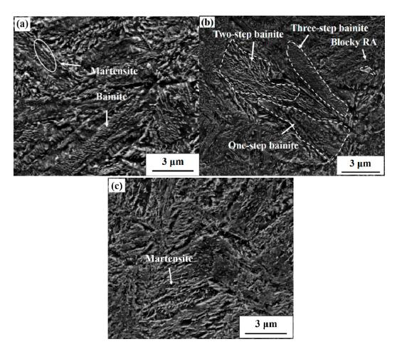
**Figure 3.** Scanning electron microscopy (SEM) micrographs of different heat treatment samples: (**a**) B1; (**b**) B3; (**c**) Q&T.
