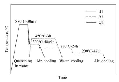
Figure 1. The schematic illustration of different heat treatments.
