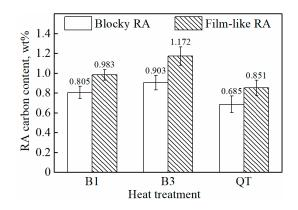
**Figure 7.** Carbon content of blocky and film-like retained austenite in the different heat treatment samples.
