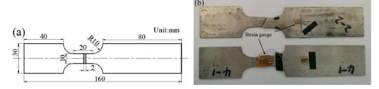
**Figure 2.** (a) Schematic illustration of heat treatment and the dynamic tensile test sample and (b) specimens attached with strain gages.
