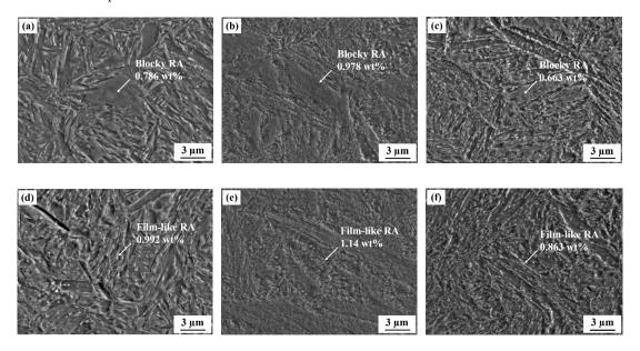
**Figure 8.** Examples showing how the carbon content of film-like and blocky retained austenite is determined: (**a**) and (**d**) for B1; (**b**) and (**e**) for B3; (**c**) and (**f**) for Q&T.
