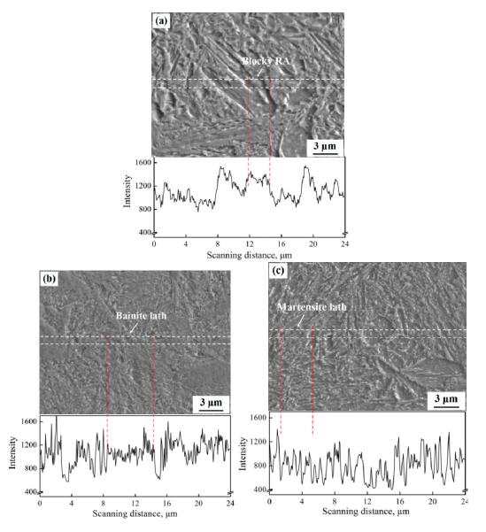
Figure 6. Line scanning of carbon element with different heat treatment samples: (a) B1; (b) B3; (c) Q&T.
