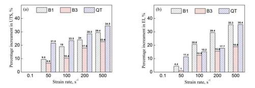
**Figure 10.** The percentage increment in (**a**) the ultimate tensile strength (UTS) and (**b**) total elongation (EI) with different heat treatments compared to the value under  $0.1 \text{ s}^{-1}$  strain rate.
