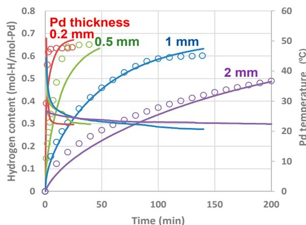
**Figure 13.** Experimental results (blank circles) and calculation fittings (solid lines) of time evolution of hydrogen content in Pd plates of various thicknesses. The single set of parameters  $k_{sb}^0 = 5.8 \times 10^{12} \text{ s}^{-1}$  and  $k_{bs}^0 = 7.6 \times 10^{11} \text{ s}^{-1}$  was used for all the calculations.
