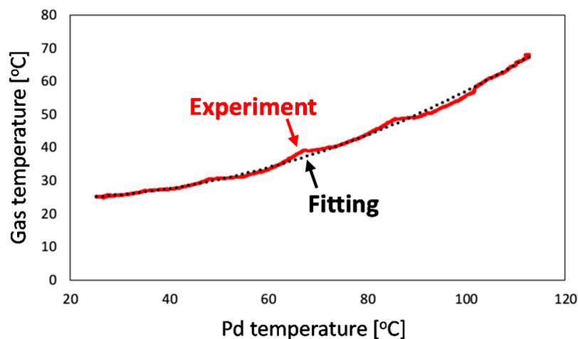
**Figure 11.** Relationship between Pd and gas phase temperatures.
