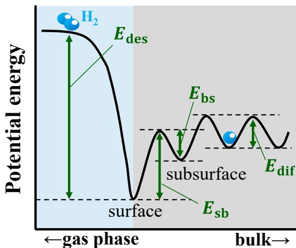
**Figure 2.** Schematic diagram of potential energy profile of hydrogen absorbing metals.  $E_{des}$ ,  $E_{sb}$ ,  $E_{bs}$ , and  $E_{dif}$  are the activation energy values for the desorption, migration of hydrogen from the surface to the subsurface and from the subsurface to the surface, and diffusion of hydrogen in the bulk region, respectively.
