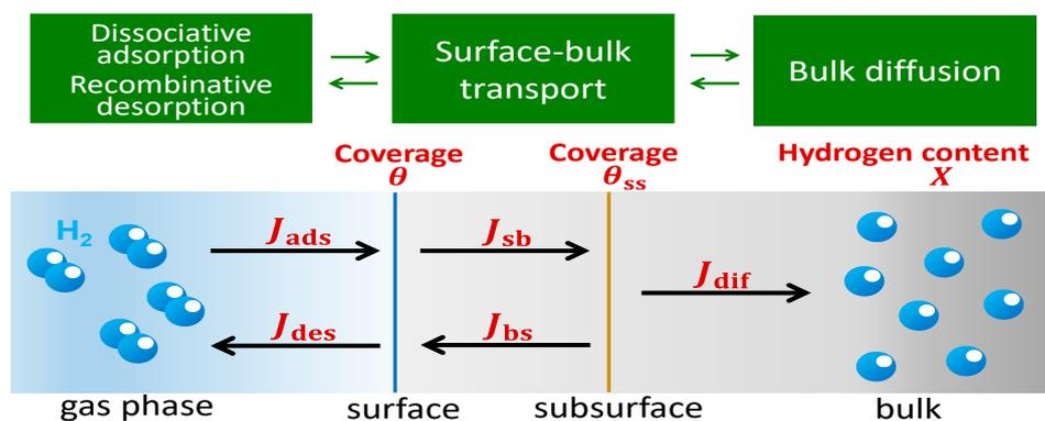
**Figure 1.** Conceptual schematic diagram of hydrogen absorption into metals.  $J_{ads}$  and  $J_{des}$  are the hydrogen fluxes for the surface adsorption and desorption processes, respectively;  $J_{sb}$  and  $J_{bs}$  are the fluxes for the migration of hydrogen from the surface to the subsurface, and from the subsurface to the surface, respectively; and  $J_{dif}$  is the hydrogen flux for the diffusion in the bulk region.
