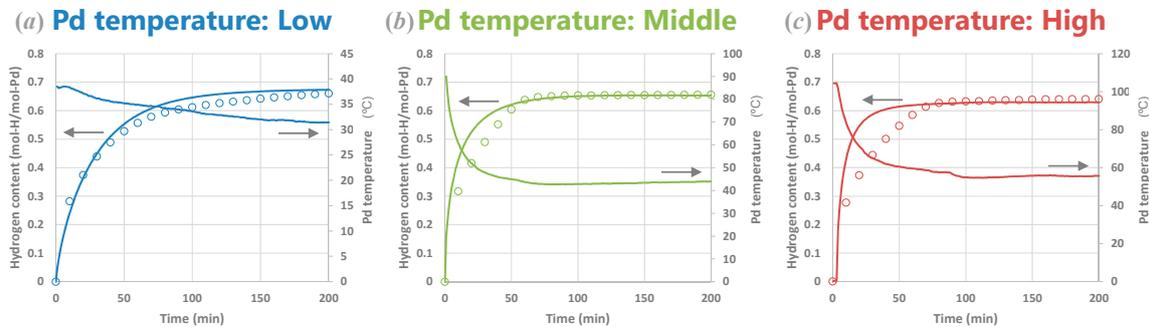
**Figure 12.** Experimental results (blank circles) and numerical fitting (solid lines) of time evolution of hydrogen content in Pd at different temperatures (*a*: low, *b*: middle, and *c*: high temperature ranges). The fitting parameters were  $k_{sb}^0 = 5.8 \times 10^{12} \text{ s}^{-1}$  and  $k_{bs}^0 = 7.6 \times 10^{11} \text{ s}^{-1}$  for all the calculations.
