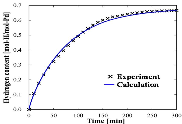
**Figure 3.** Experimental result and calculated fitted result of the time evolution of hydrogen content in Pd at 17 °C.
