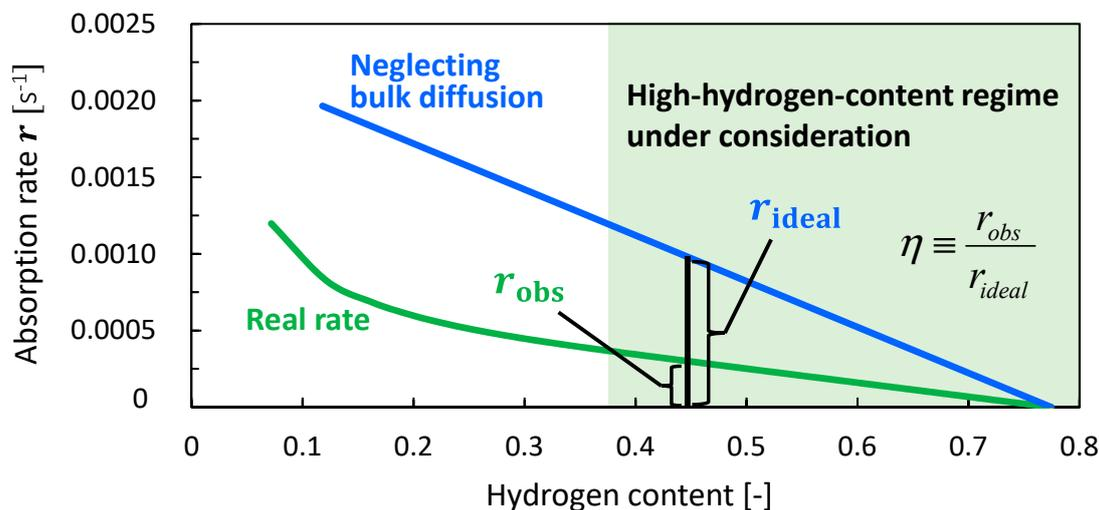
**Figure 14.** Conceptual schematic for definition of effectiveness factor  $\eta$ ;  $\eta = r_{obs}/r_{ideal}$ , where  $r_{obs}$  and  $r_{ideal}$  are the actually observed hydrogen absorption rate that accounts for bulk diffusion and the virtual absorption rate that was calculated neglecting the bulk diffusion process.  $r_{obs}$  and  $r_{ideal}$  were plotted against the hydrogen content.
