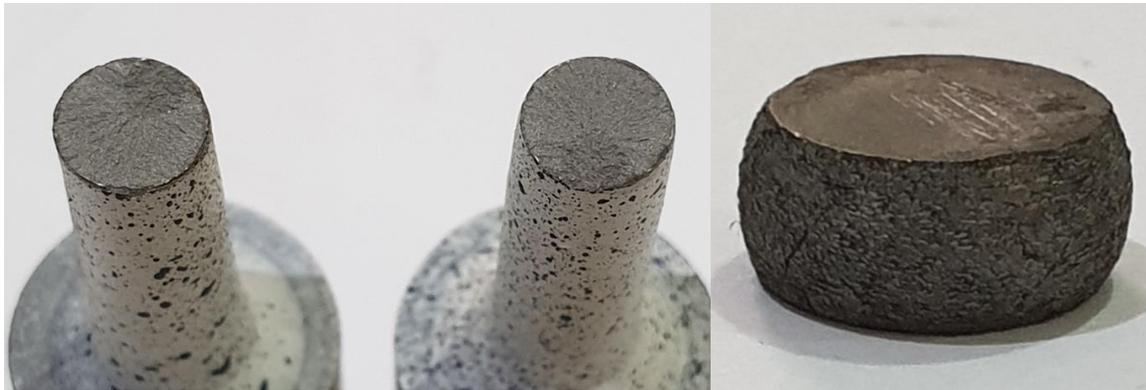
**Figure 7.** A flat fracture mode surface for “D2” tool steel under tension (**left**) and flattened shape of the cylindrical specimen (**right**) under compression.
