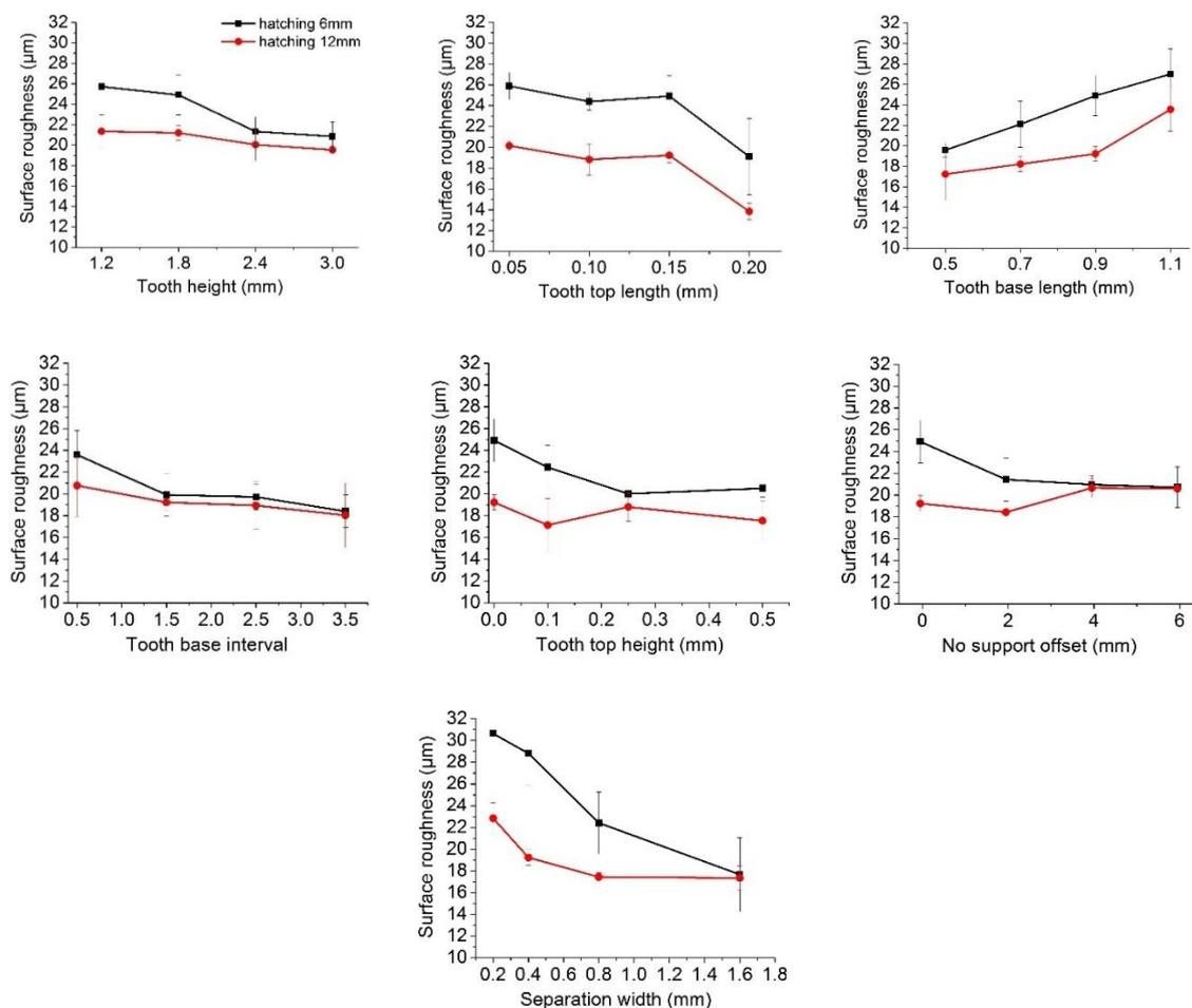
**Figure 12.** Effect of support parameters on surface roughness.
