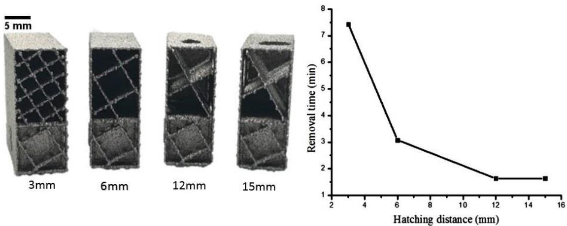
Figure 8. Effect of hatching distance on support removability.
