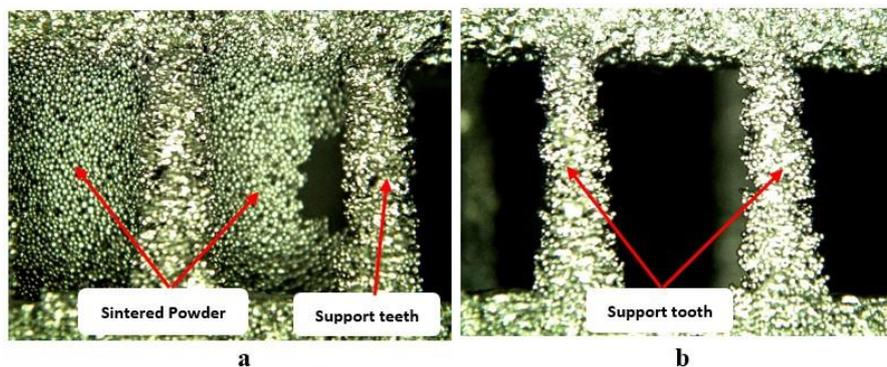
**Figure 5.** Support tooth structures: (a) before powder removal; (b) after powder removal.
