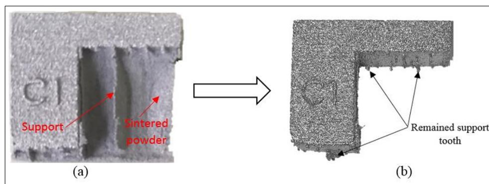
**Figure 11.** Specimen C1 (current = 1.25 mA) (a) before powder-blasting process, and (b) after powder-blasting process.
