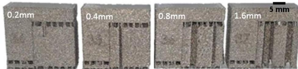
**Figure 9.** Support structures with various fragmentation separation widths.
