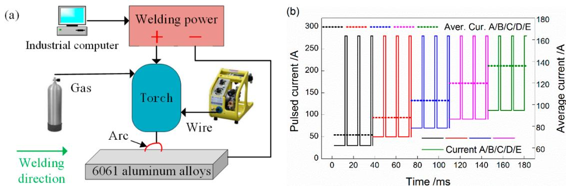
**Figure 1.** Schematic of (a) experimental setup and (b) the adjustment of average current.
