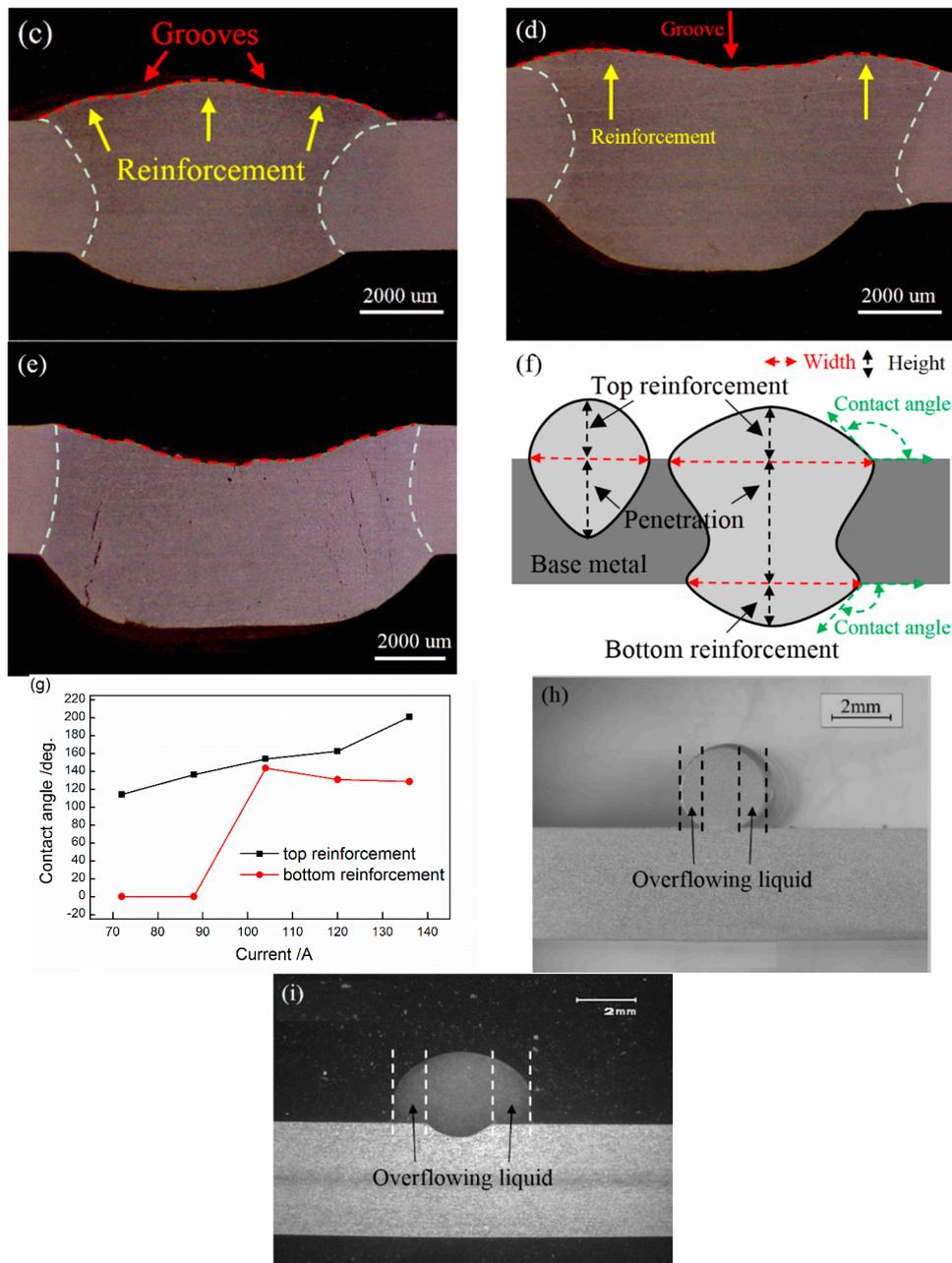
**Figure 2.** Profiles of weld bead and its dimensions. (a) 72 A; (b) 88 A; (c) 104 A; (d) 120 A; (e) 136 A; (f) schematic of measurement; (g) contact angle; (h) bead of CMT + P (reproduced from [7], with permission of Elsevier, 2016); and (i) bead of TIG-CMT (reproduced from [12], with permission of Elsevier, 2017).
