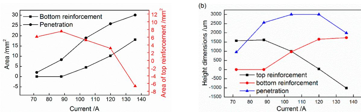
**Figure 3.** Dimensions of beads welded with different average currents. (a) Area of different parts. (b) Height of different parts.
