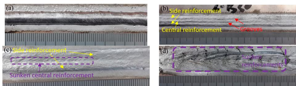
**Figure 4.** Appearances of the top surface for bead welded with different average current. (a) Less than 88A; (b) 104 A; (c) 120 A; (d) 136 A.
