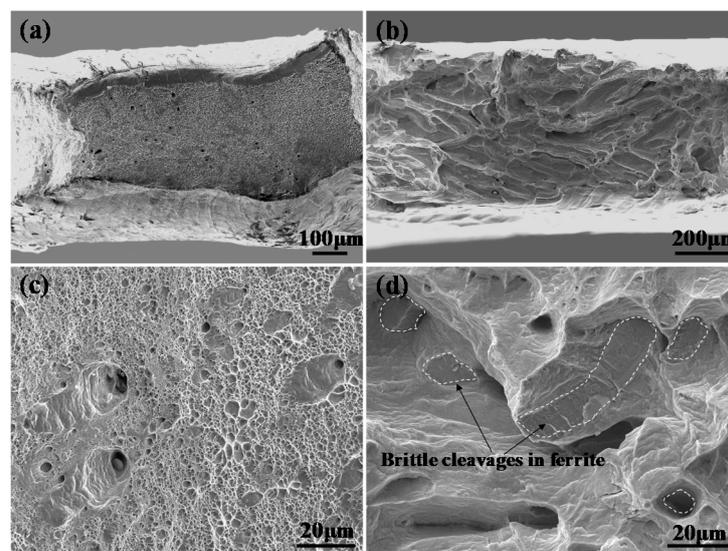
**Figure 3.** (a,c) Macroscopic and microscopic morphologies of the fracture surface of the un-aged CDSS (b,d) and of the long-term thermally aged CDSS.
