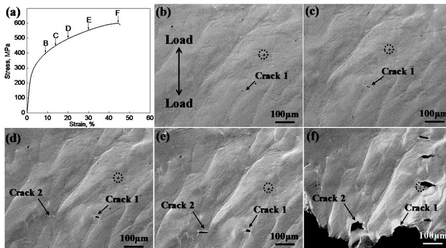
**Figure 4.** (a) In situ observation at different stages for strains (b)  $\epsilon = 9\%$ ; (c) 14%; (d) 20%; (e) 30%; and (f) rupture of CDSS thermally aged at 400 °C for 20,000 h. An inclusion is marked by a dashed circle as the position mark.
