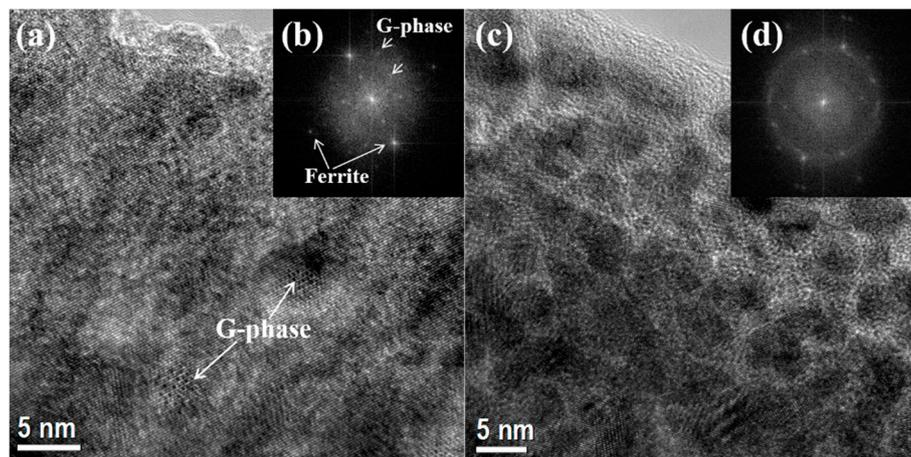
**Figure 6.** (a) HRTEM images of ferrite in the undeformed and (c) deformed samples of the steels thermally aged at 400 °C for 20,000 h. (b) and (d) are the corresponding FFT patterns of (a) and (c), respectively.
