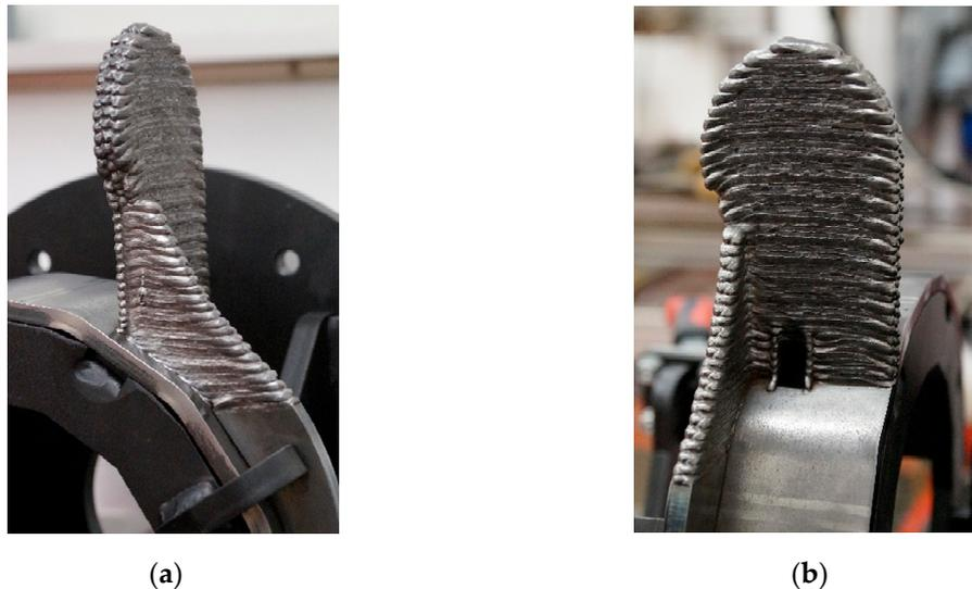
**Figure 12.** (a) Result of the first attempt for manufacturing the AM-part; (b) detailed view of the featured cut-out.
