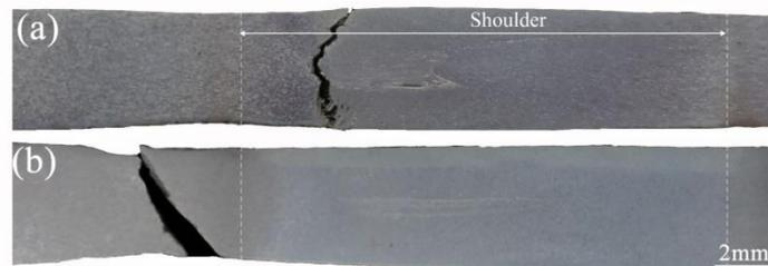
**Figure 12.** Typical fracture location of joints at different rotation speeds: (a) 600 r/min; (b) 800 r/min.
