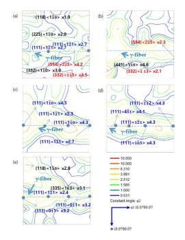
**Figure 8.**  $\varphi_2 = 45^\circ$  section of the ODF in the alloy B steel specimens heat-treated under different conditions: (**a**) as-received, (**b**) 800 °C, 6 min, (**c**) 1050 °C, 6 min, and 800 °C, 6 min, (**d**) 1050 °C, 30 min, and 800 °C, 6 min, and (**e**) 1150 °C, 6 min, and 800 °C, 6 min.
