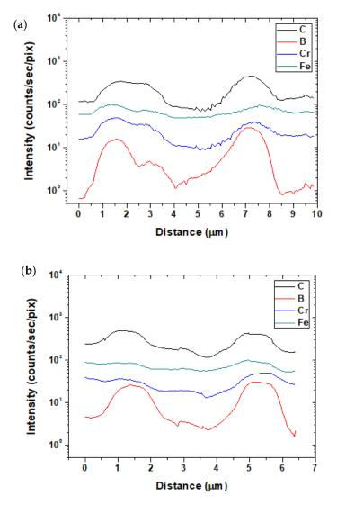
**Figure 14.** Nano-SIMS distribution map of sputtered carbon, boron, chromium, and iron ions in the areas denoted by the arrows of the alloy B specimens heat-treated under the 1050 °C, 6 min and 800 °C, 6 min conditions: (**a**) #1 (**b**) #2.
