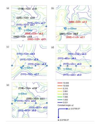
**Figure 9.**  $\varphi_2 = 45^\circ$  section of the ODF of the Gr.92 steel specimens heat-treated under different conditions: (a) as-received, (b) 800 °C, 6 min, (c) 1050 °C, 6 min, and 800 °C, 6 min, (d) 1050 °C, 30 min, and 800 °C, 6 min, and (e) 1150 °C, 6 min, and 800 °C, 6 min.
