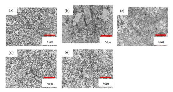
**Figure 4.** Optical microscope (OM) images of the alloy B steel specimens subjected to different intermediate heat treatment conditions: (**a**) as-received; (**b**) 800 °C, 6 min; (**c**) 1050 °C, 6 min and 800 °C, 6 min; (**d**) 1050 °C, 30 min, and 800 °C, 6 min; (**e**) 1150 °C, 6 min, and 800 °C, 6 min.
