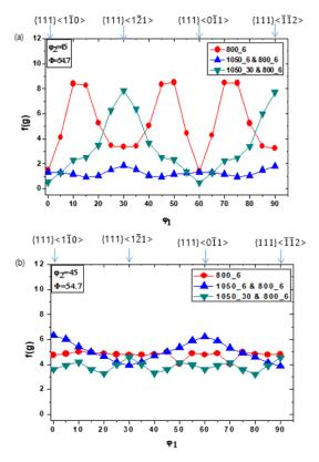
**Figure 10.** Evolution of the ODF intensity f(g) in the  $\gamma$ -fiber ( $\Phi = 54.7^{\circ}$  and  $\varphi_2 = 45^{\circ}$ , constant) components of the steels subjected to different intermediate heat treatment conditions: (**a**) alloy B and (**b**) Gr.92.
