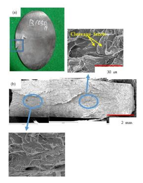
**Figure 3.** Alloy B steel during the rolling process under the tempering condition after the normalization: (a) fractograph of failed part and (b) scanning electron microscopy (SEM) image.
