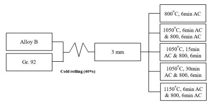
Figure 1. Schematic of the experimental procedure. AC: air cooling.
