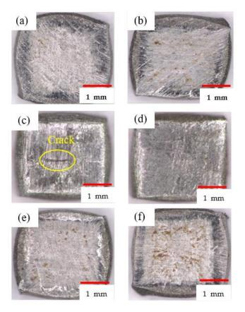
**Figure 12.** Images of the specimens heat-treated under different conditions after the compression test along the ND: (**a**) alloy B 800 °C, 6 min, (**b**) Gr.92 800 °C, 6 min, (**c**) alloy B 1050 °C, 6 min, and 800 °C, 6 min (**d**) Gr.92 1050 °C, 6 min, and 800 °C, 6 min, (**e**) alloy B 1150 °C, 6 min, and 800 °C, 6 min, and (**f**) Gr.92 1150 °C, 6 min, and 800 °C, 6 min.
