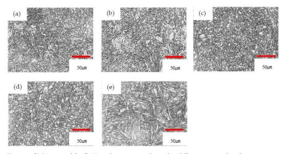
**Figure 5.** OM images of the Gr.92 steel specimens subjected to different intermediate heat treatment conditions: (**a**) as-received; (**b**) 800 °C, 6 min; (**c**) 1050 °C, 6 min, and 800 °C, 6 min; (**d**) 1050 °C, 30 min, and 800 °C, 6 min; (**e**) 1150 °C, 6 min, and 800 °C, 6 min.
