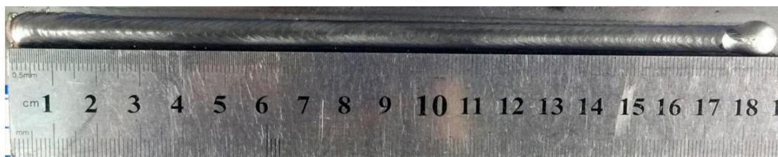
**Figure 12.** The morphology of the weld bead using optimal parameters combination.
