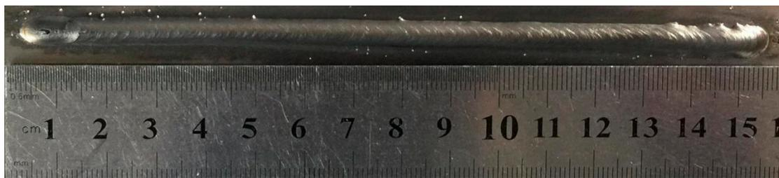
**Figure 11.** The appearance of the weld bead using optimal parameters combination.
