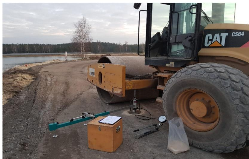
**Figure 9.** Measurement of base course bearing capacity in the field (J. Krasowski).
