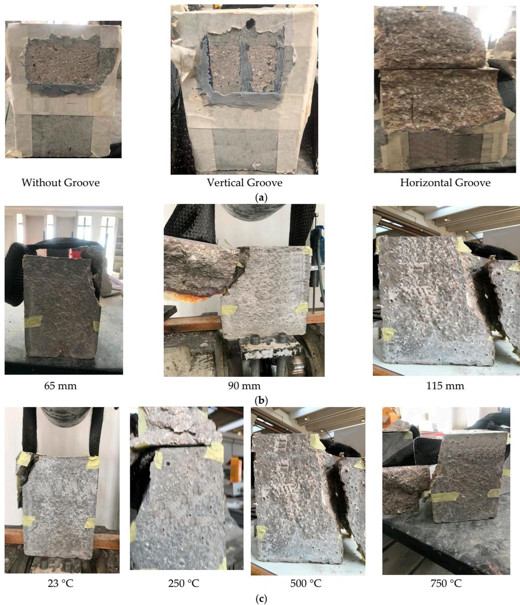
**Figure 5.** Typical mode of failure. (a) Specimens with different drilling diameters; (b) specimens with different CFRP bonded lengths; (c) specimens with different temperature degrees.
