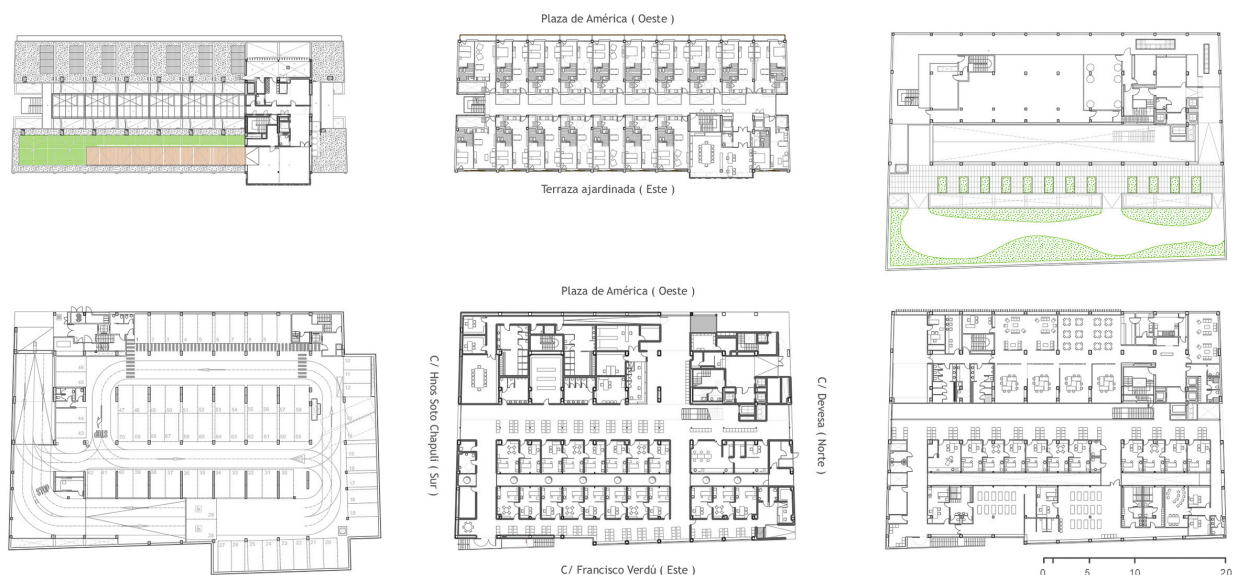
Figure 11. Plaza de América building: floor plans. Clockwise from upper left corner: seventh floor (sun deck and common facilities); levels 3–6 (typical housing unit floor plan); second floor (services, gardens and urban orchard); first floor (community health center and day care center); ground floor (community health center and main access); –1, –2 & –3 basement levels (parking). Courtesy of Carmen Pérez Molpeceres and Consuelo Argüelles Álvarez.
