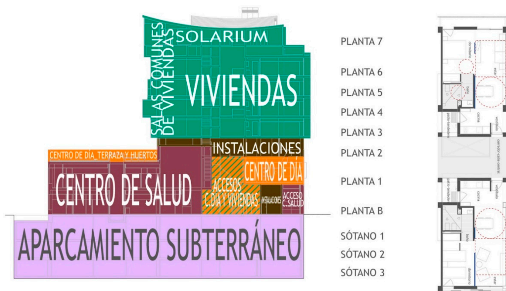
Figure 13. Cross-section diagram of the Plaza de América building (from bottom to top: −1, −2 & −3 basement levels: parking; ground floor: community health center and main access; first floor: community health center and day care center; second floor: services, gardens and urban orchard; levels 3 to 6: dwellings and collective areas; seventh floor: sun deck and common facilities) and typical housing unit floorplan. Courtesy of Carmen Pérez Molpeceres and Consuelo Argüelles Álvarez.
