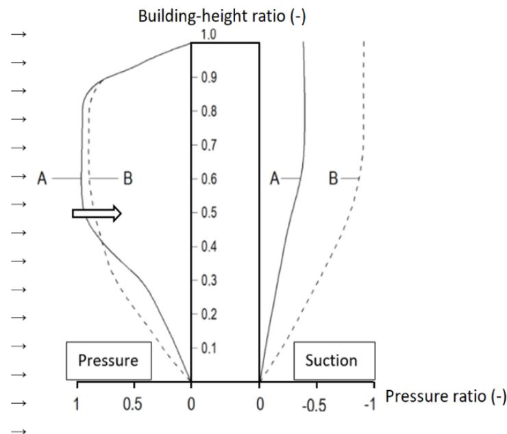
**Figure 1.** The approximate influence of the facade air permeability on the pressure and suction distribution on windward and leeward side for tall building with rectangular ground plan, A—zero air permeability building, B—air permeability building, (source authors, processed according to [11]).
