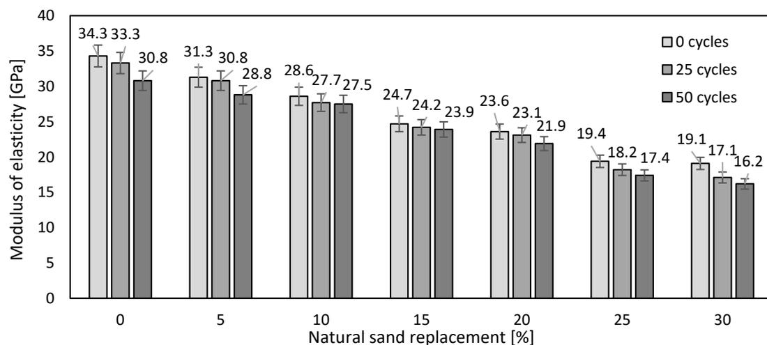
Figure 7. Dynamic modulus of elasticity during freezing-thawing.
