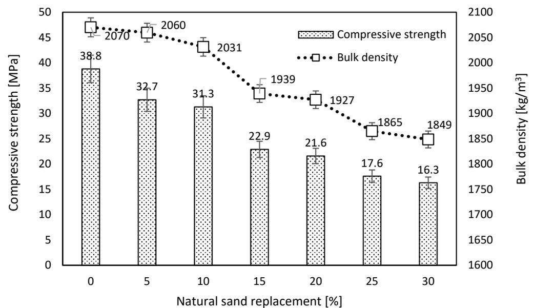
Figure 5. Compressive strength and bulk density after 28 days.
