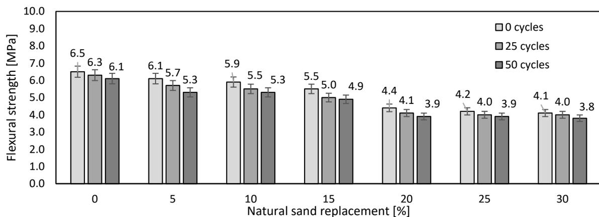
Figure 8. Flexural strength during freezing–thawing.
