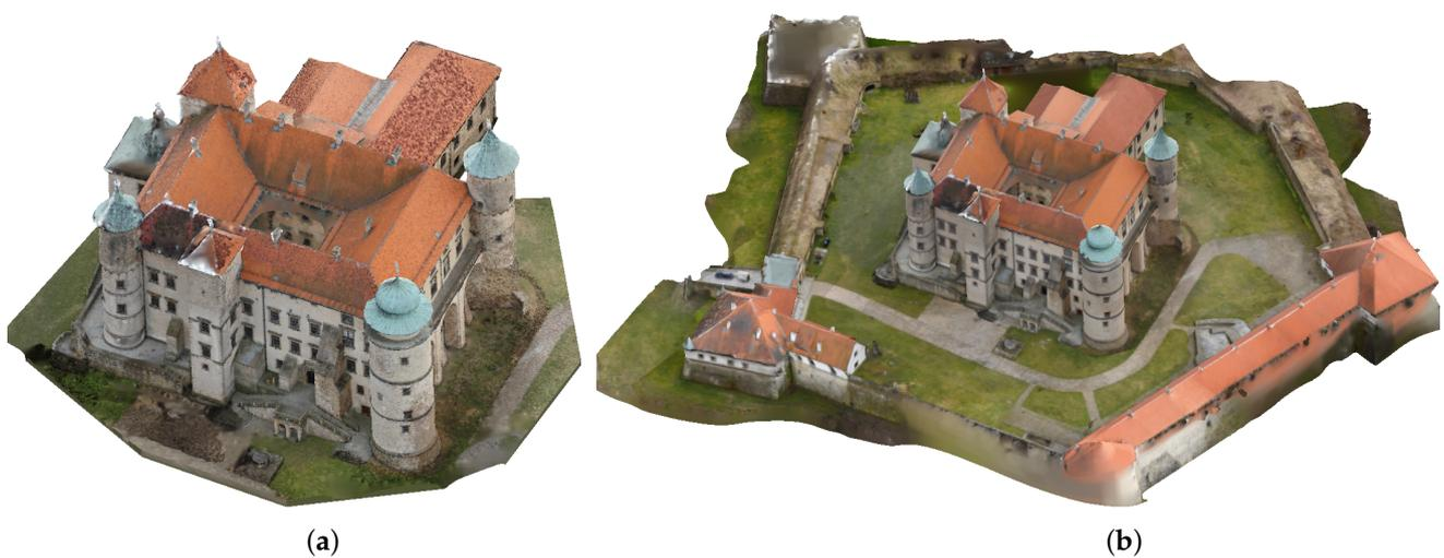
**Figure 14.** Polygon models of the castle in Nowy Wiśnicz: only the building (4,133,352 faces) (a); the building with fortifications (1,966,487 faces) (b).
