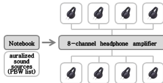
**Figure 8.** Equipment configuration diagram for the speech intelligibility test.
