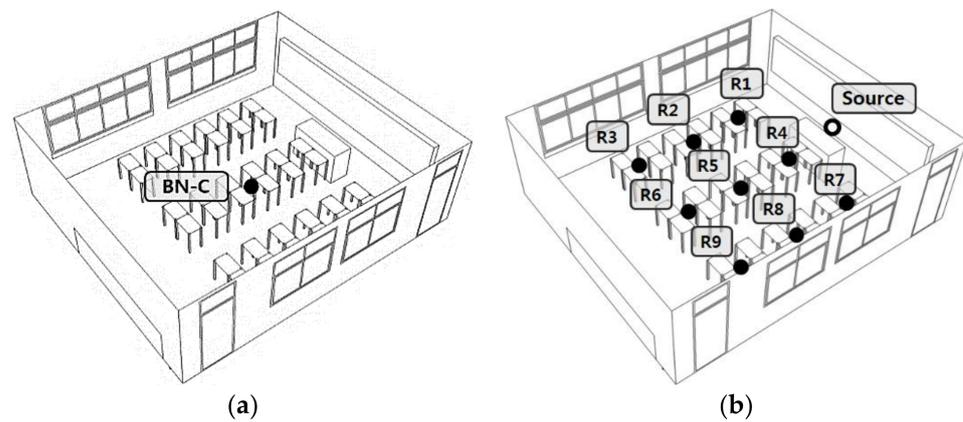
**Figure 1.** The location of sound sources and receiving points for measurements in the classroom. (a) Background noise level; (b) reverberation time,  $T_{30}$ .
