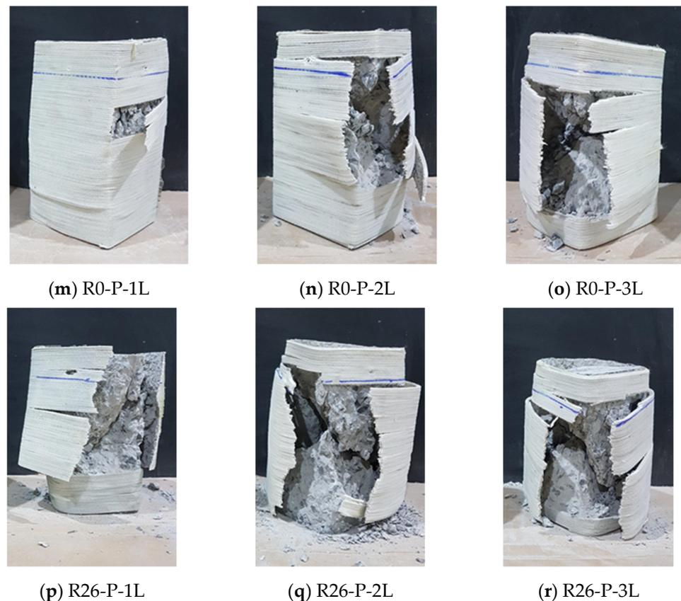
**Figure 6.** Ultimate failures of FRRP-confined specimens.
