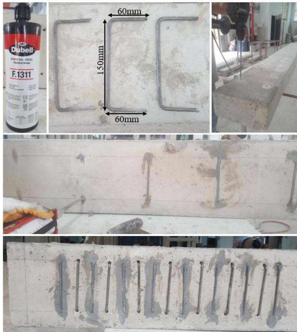
Figure 2. Strengthening beams with MSS.
