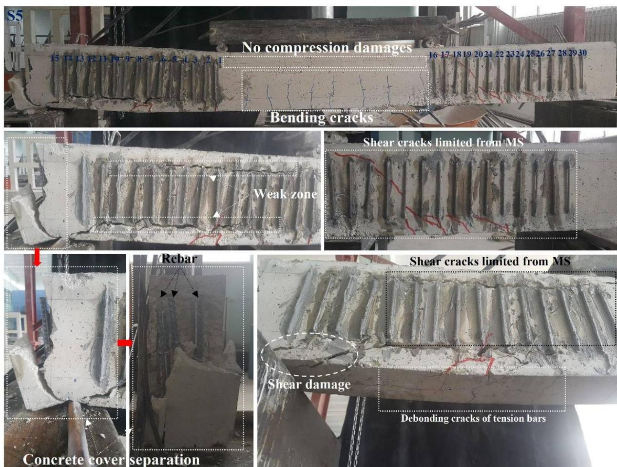
Figure 12. Damages at S5.
