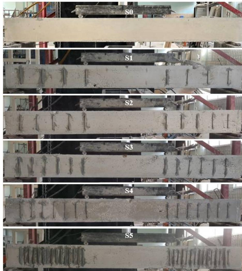
Figure 5. Pre-experiment view of reference and reinforced beams.
