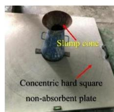
(a) Placement of slump cone
