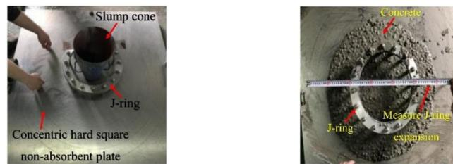
(a) Placement of slump cone and J-ring (b) Measure and count
