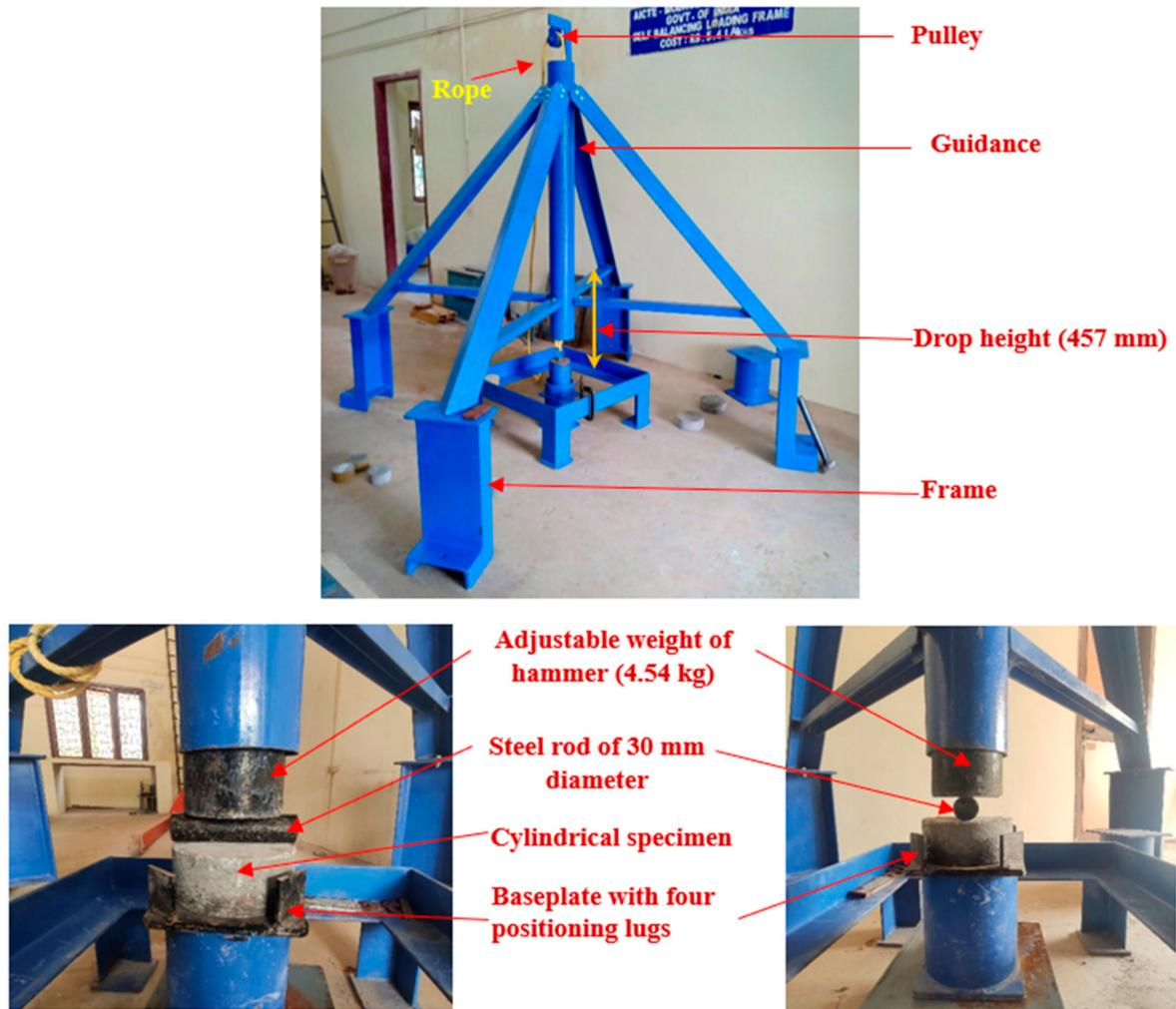
**Figure 8.** Device for measuring the impact of falling masses at low velocity.
