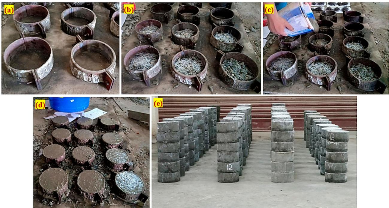
**Figure 7.** Casting procedure: (a) empty mold, (b) filling the mold with premixed fibers and coarse aggregate, (c) grout pouring process, (d) specimen appearance after casting, and (e) after demolding, where the specimens were left on the floor.
