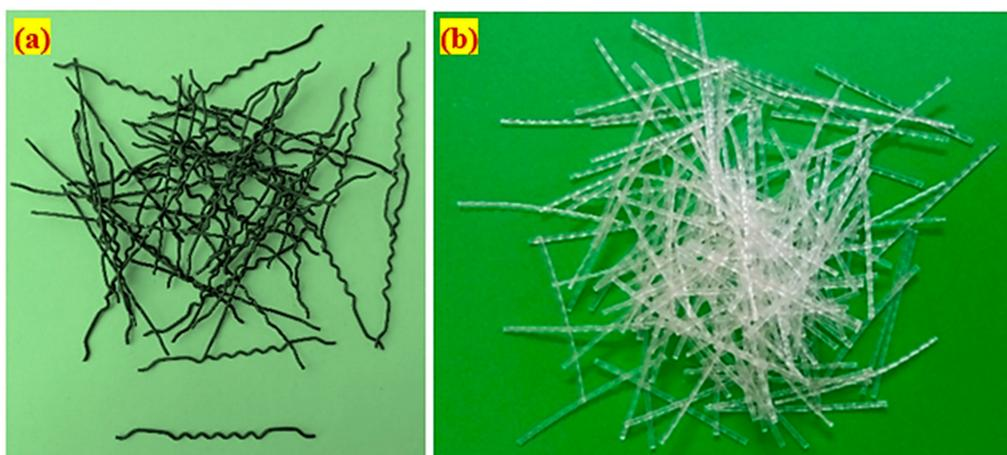
**Figure 5.** Fiber appearance: (a) hybrid shape of hooked-end crimped and (b) macro polypropylene fiber.
