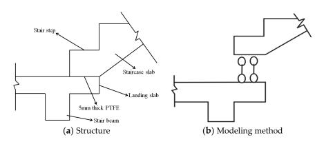
and the reinforcement was the 2-node 3-dimensional truss element (T3D2). The models are in Figure 2.
