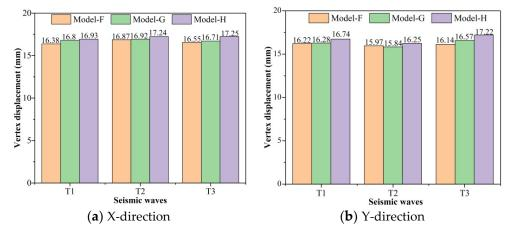
Figure 21. The maximum vertex displacement of the models.
