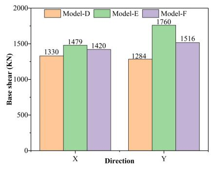
Figure 11. Aa comparison of max base shear of models.
