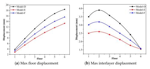
Figure 10. The floor displacement and interlayer displacement in the Y-direction.
