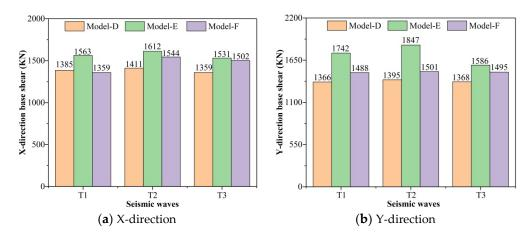
Figure 14. A comparison of the max base shear of the models.
