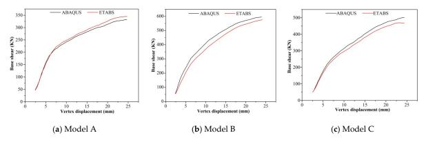
Figure 4. The base shear-vertex displacement curves.
