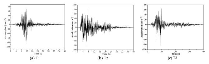
Figure 13. The time-history curves of the seismic waves.
