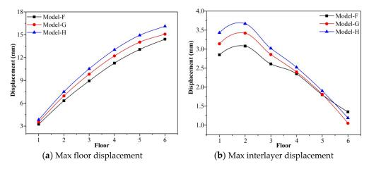
Figure 18. The floor displacement and interlayer displacement in the X-direction.
