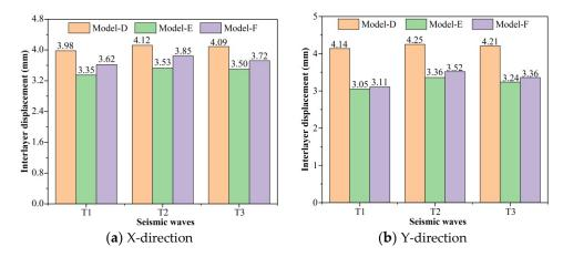
Figure 16. A comparison of the maximum interlayer displacement of the models.
