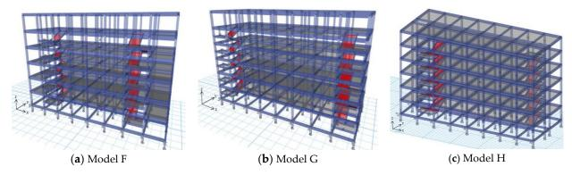
Figure 7. The models of three different staircase positions.
