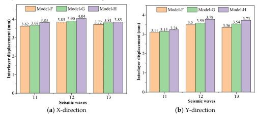
Figure 22. The maximum interlayer displacement of the models.
