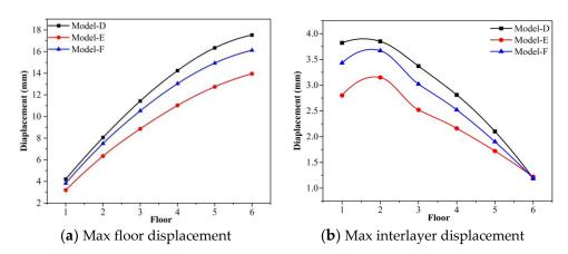
Figure 9. The floor displacement and interlayer displacement in the X-direction.
