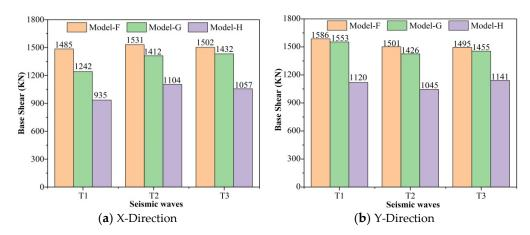
Figure 20. The maximum base shear of the models.
