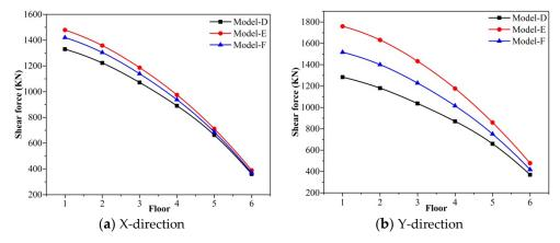
Figure 12. A comparison of the max interlayer shear forces of the models.
