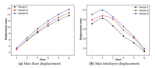
Figure 19. The floor displacement and interlayer displacement in the Y-direction.
