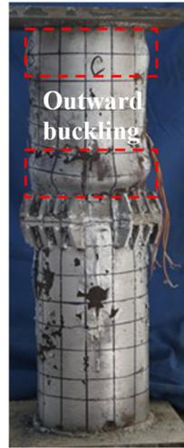
**Figure 5.** Failure mode of BWCFSST short column specimen without imperfection.
